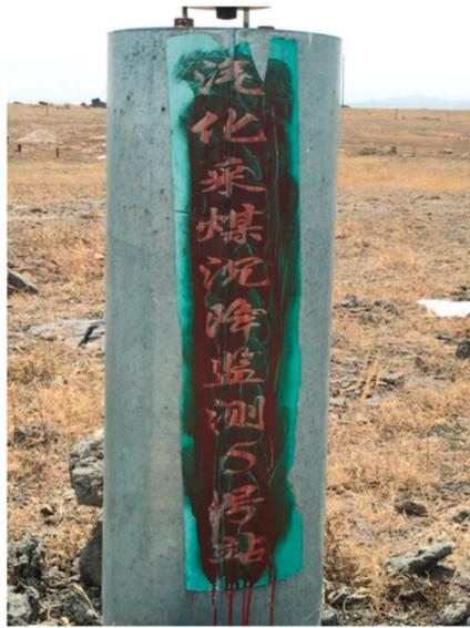
**Figure 11.** UCG surface subsidence No. 5 monitoring station.
