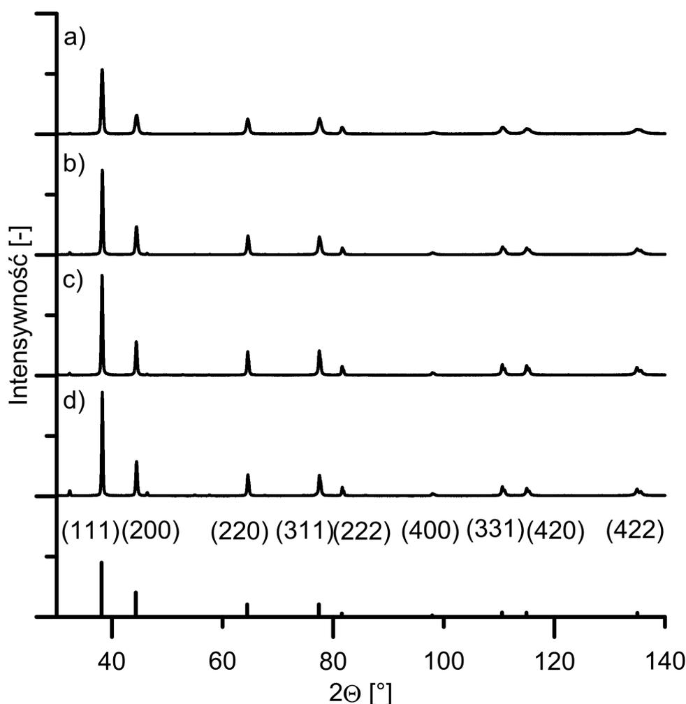
**Figure 2.** XRD patterns of the silver structures prepared in the conventional heating process, reductant (a) 1,3-butanediol or (b) 1,3-propanediol, and a microwave-assisted process, reductant (c) 1,3-butanediol or (d) 1,3-propanediol.
