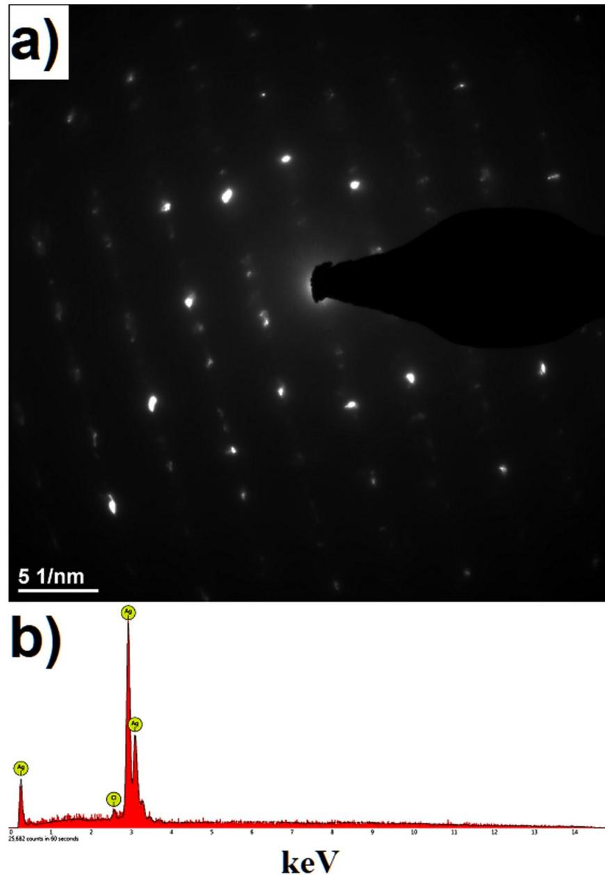
**Figure 5.** Silver nanowires synthesised in the microwave-assisted process, 1,3-propanediol reducer: (a) SAED pattern of AgNWs, (b) EDS spectrum for AgNWs.
