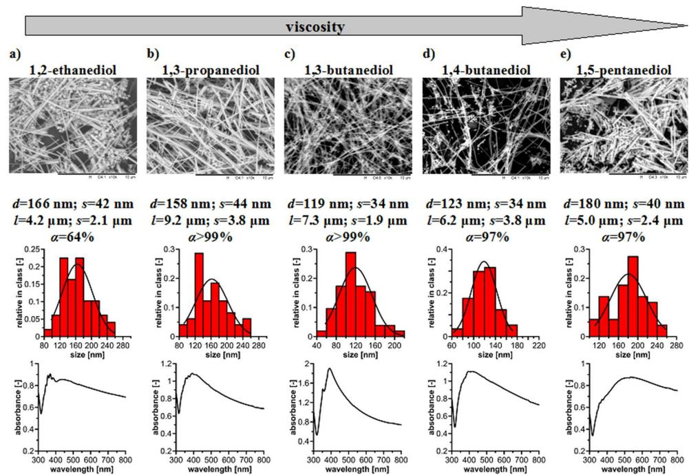
**Figure 6.** A summary of the properties of AgNWs produced with the application of the different reductants in a batch process under conventional heating conditions: (a) 1,2-ethanediol, (b) 1,3-propanediol, (c) 1,3-butanediol, (d) 1,4-butanediol, (e) 1,5-pentanediol.  $d$ ,  $l$ —average diameter, length, respectively;  $s$ —standard deviation,  $\alpha$ —conversion; scale bar 10  $\mu\text{m}$ .
