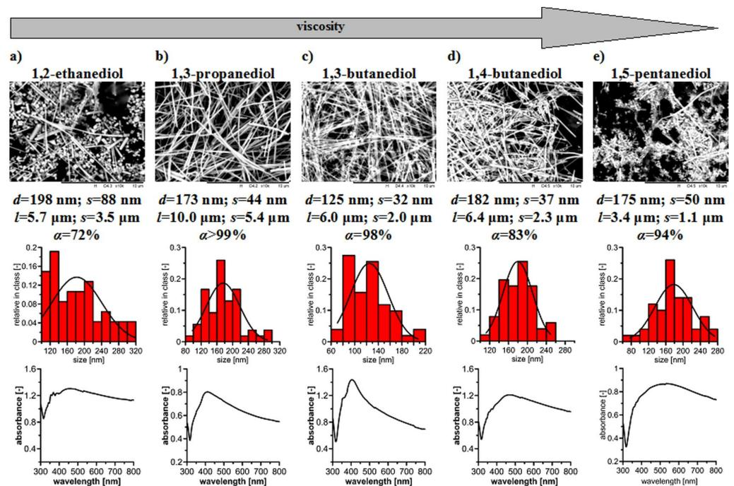
**Figure 7.** A summary of the properties of AgNWs produced with the application of the different reductants in a batch, microwave-assisted process: (a) 1,2-ethanediol, (b) 1,3-propanediol, (c) 1,3-butanediol, (d) 1,4-butanediol, (e) 1,5-pentanediol.  $d$ ,  $l$ —average diameter, length, respectively;  $s$ —standard deviation;  $\alpha$ —conversion; scale bar 10  $\mu\text{m}$ .
