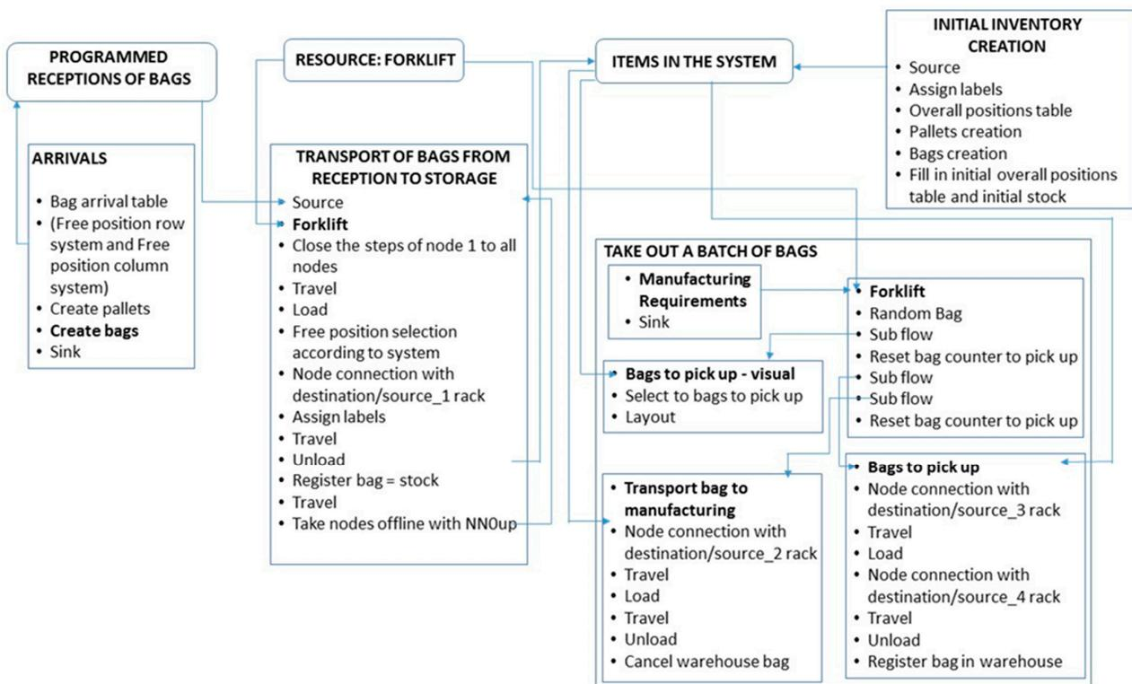
Figure 8. Scheme of the main elements of simulation model.
