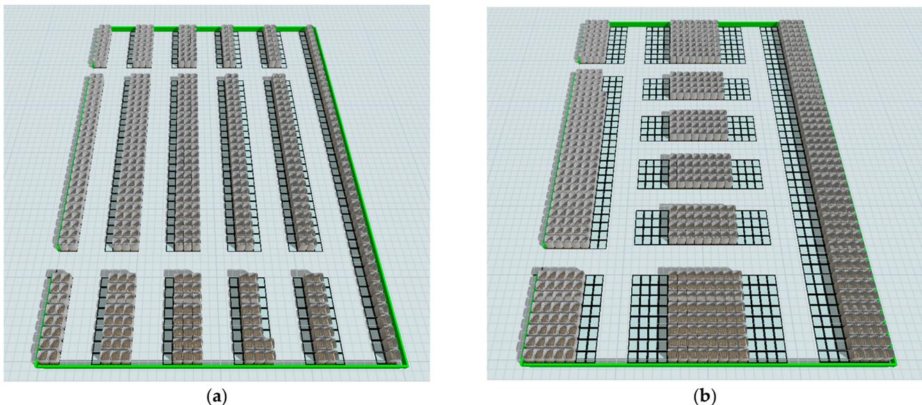
**Figure 10.** Layouts with a greater number of transversal or longitudinal zones: (a) layout ( $6 \times 3$ ) with 76.3% occupancy rate = 50% occupancy rate layout ( $3 \times 3$ ); (b) layout ( $3 \times 6$ ) with 65.0% occupancy rate = 50% occupancy rate layout ( $3 \times 3$ ).
