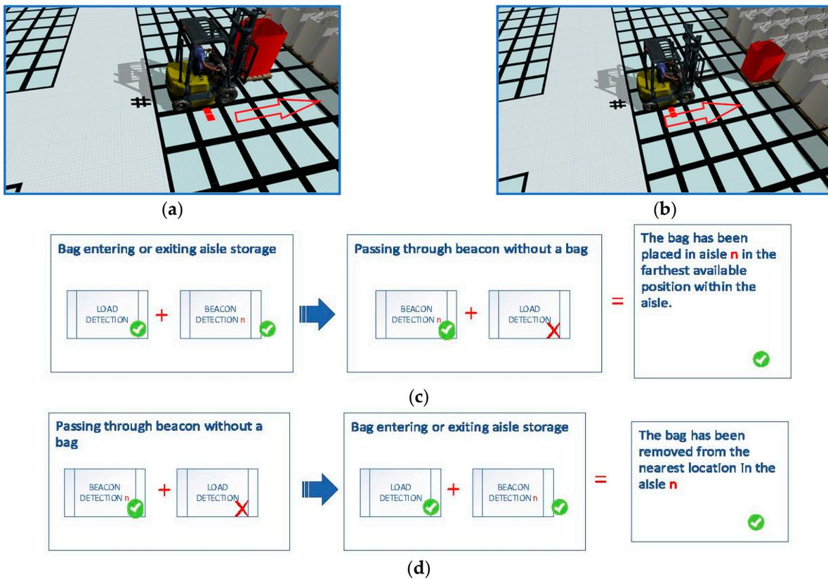
Figure 5. Sequence of the readings of RFID readers: (a) bag unloading; (b) bag extraction; (c) sequences of readings in the unloading of bags; (d) sequences of readings in the extraction of bags.
