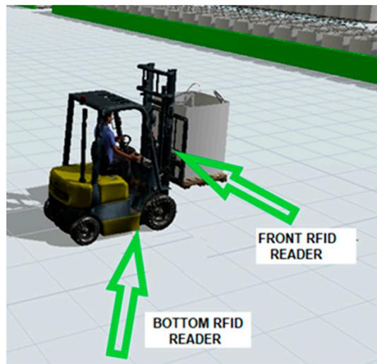
Figure 4. Forklift RFID readers.
