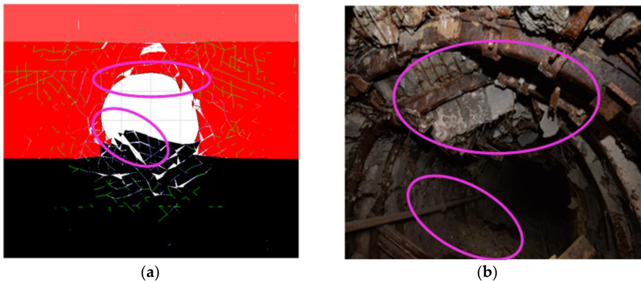
**Figure 13.** Comparison between on-site damage characteristics and simulated damage characteristics of the roadway. (a) simulated damage characteristics; (b) on-site damage characteristics.
