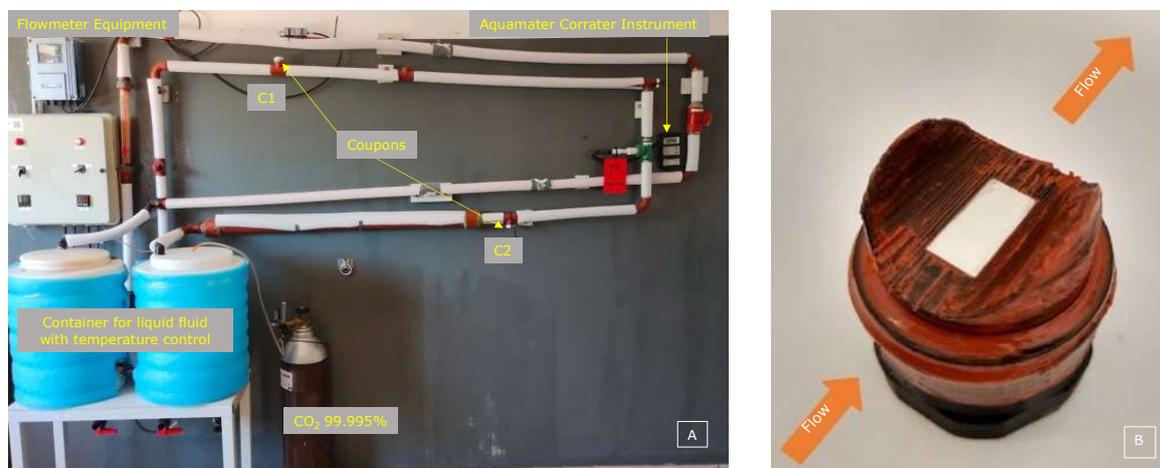
Figure 1. (A) Corrosion loop and its components; (B) coupon.
