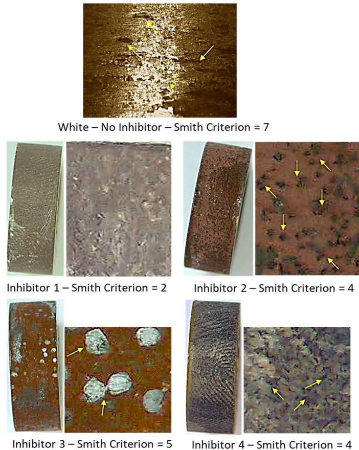
**Figure 3.** Fractographies of the tested graduated cylinders (20×). The yellow arrows show the presence of pitting according to Smith's criterion.
