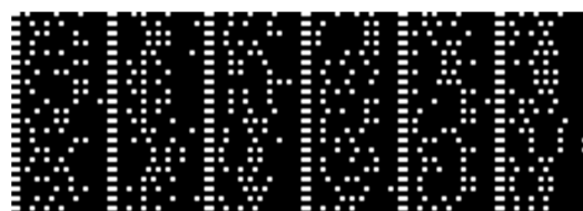
Figure 1. Binary data page of archival holographic memory.
