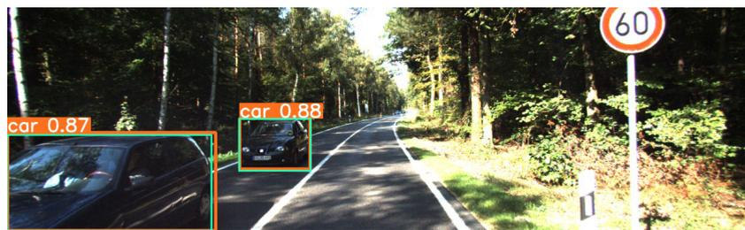
**Figure 3.** KITTI dataset image with two different bounding boxes representation: orange for the ground truth and green for the one generated with the auto-labeled model, respectively.
