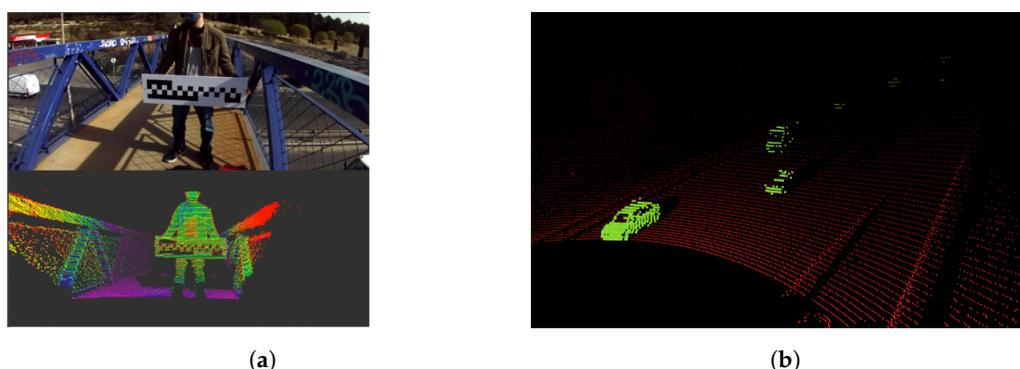
**Figure 8.** (a) Custom calibration board. (b) LiDAR view from the bridge.
