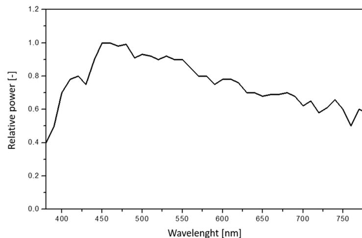
**Figure 3.** Spectral relative power distribution as a function of wavelength for the light source used.
