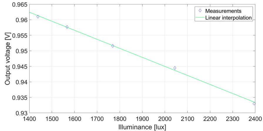
**Figure 9.** Output voltage as a function of the irradiation level.
