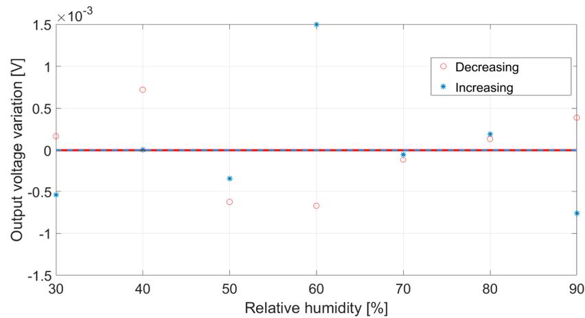
**Figure 7.** Relative humidity effects on the output voltage; the graph includes the increment and decrement of the influence applied to the plant. The  $y = 0$  line is included as a visual guide.
