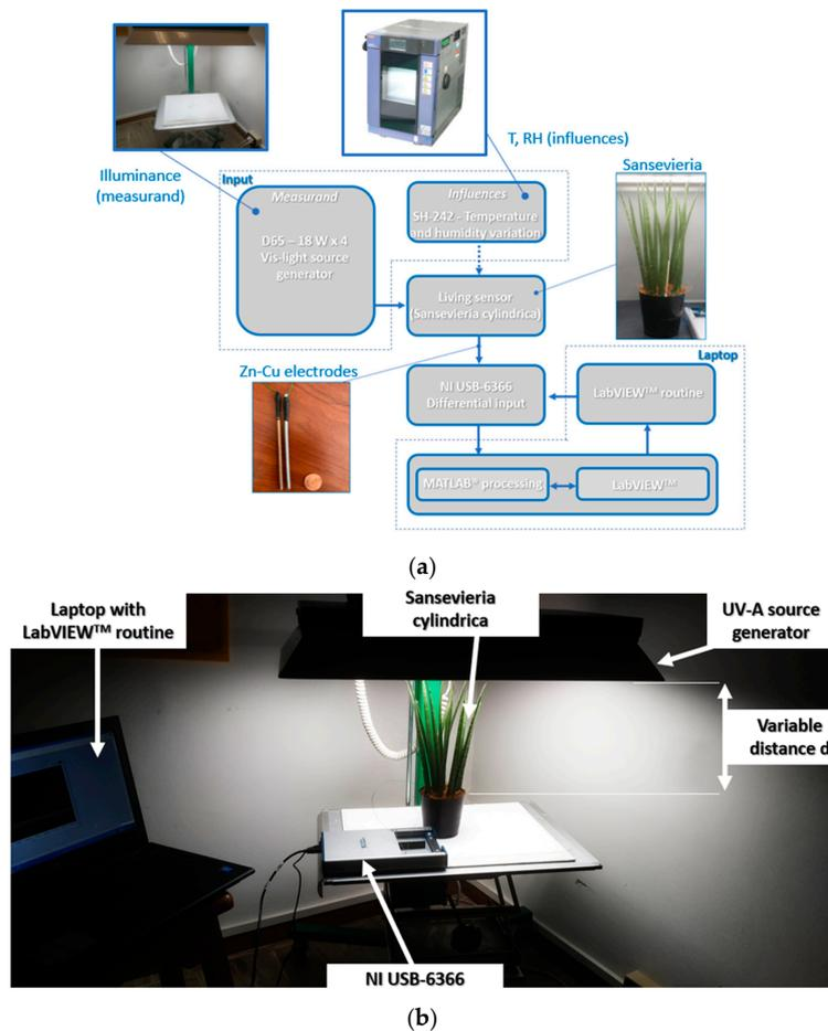
Figure 2. Block diagram of the measurement system for the characterization (a) and the experimental setup (b).
