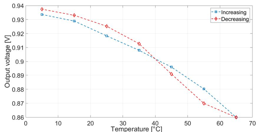
**Figure 6.** Temperature effects on the output voltage. The graph includes the increment and decrement evolution as a function of the applied influence.
