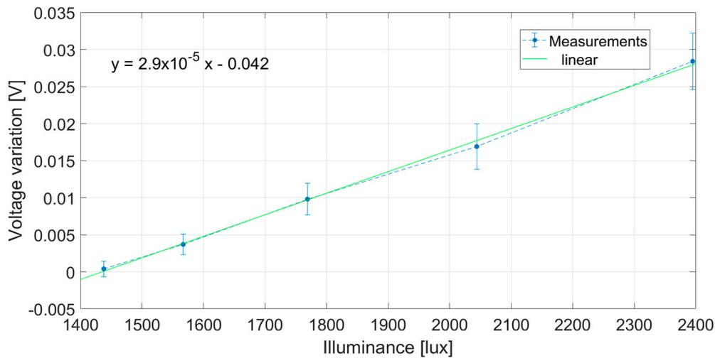
**Figure 10.** Calibration diagram of the *Sansevieria cylindrica* used as living sensor.
