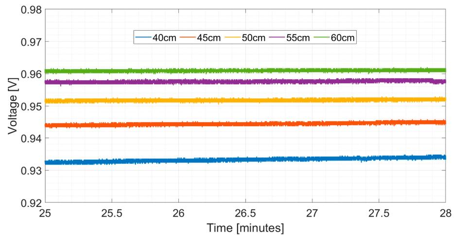
**Figure 8.** Output voltage across the electrodes as a function of the time considering various distances between plant and Vis-light source.
