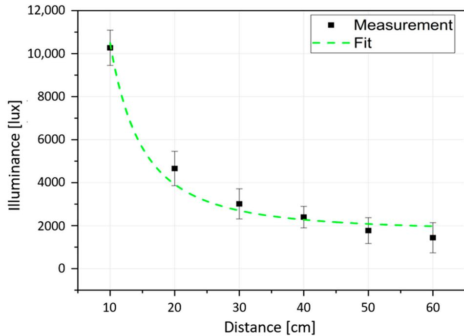
Figure 4. Illuminance level as a function of the distance  $d$  from source and detector.
