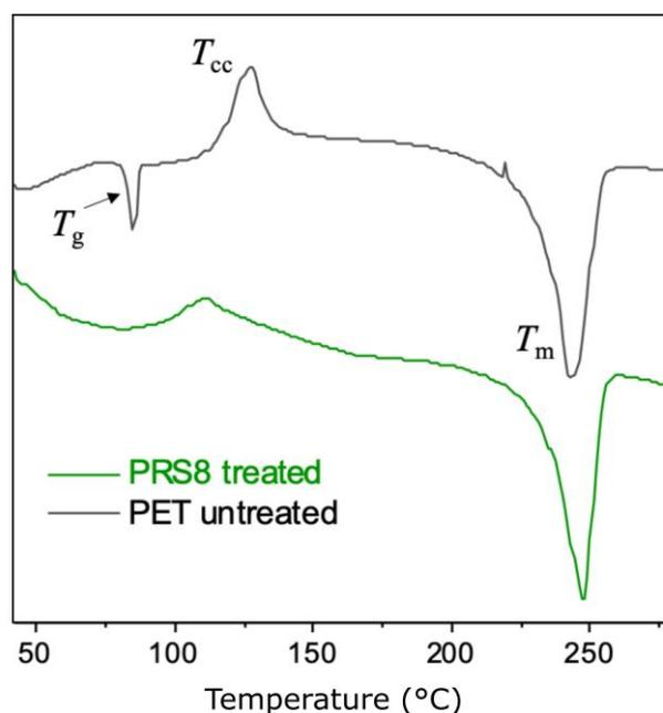
**Figure 11.** DSC heating curves (first cycle, exo up) of the untreated PET and PET treated with the extracellular fraction of *S. maltophilia* PRS8. The  $T_g$ ,  $T_{cc}$  and  $T_m$  are shown on the PET untreated curve.
