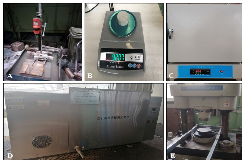
Figure 2. Actual picture of the test equipment a rock coring drilling machine (A), a high precision electronic scale (B), a programmable temperature-controlled muffle furnace (C), a rock thermal shock rupture test bench (D), a microcomputer-controlled electric-hydraulic servo press (E).
