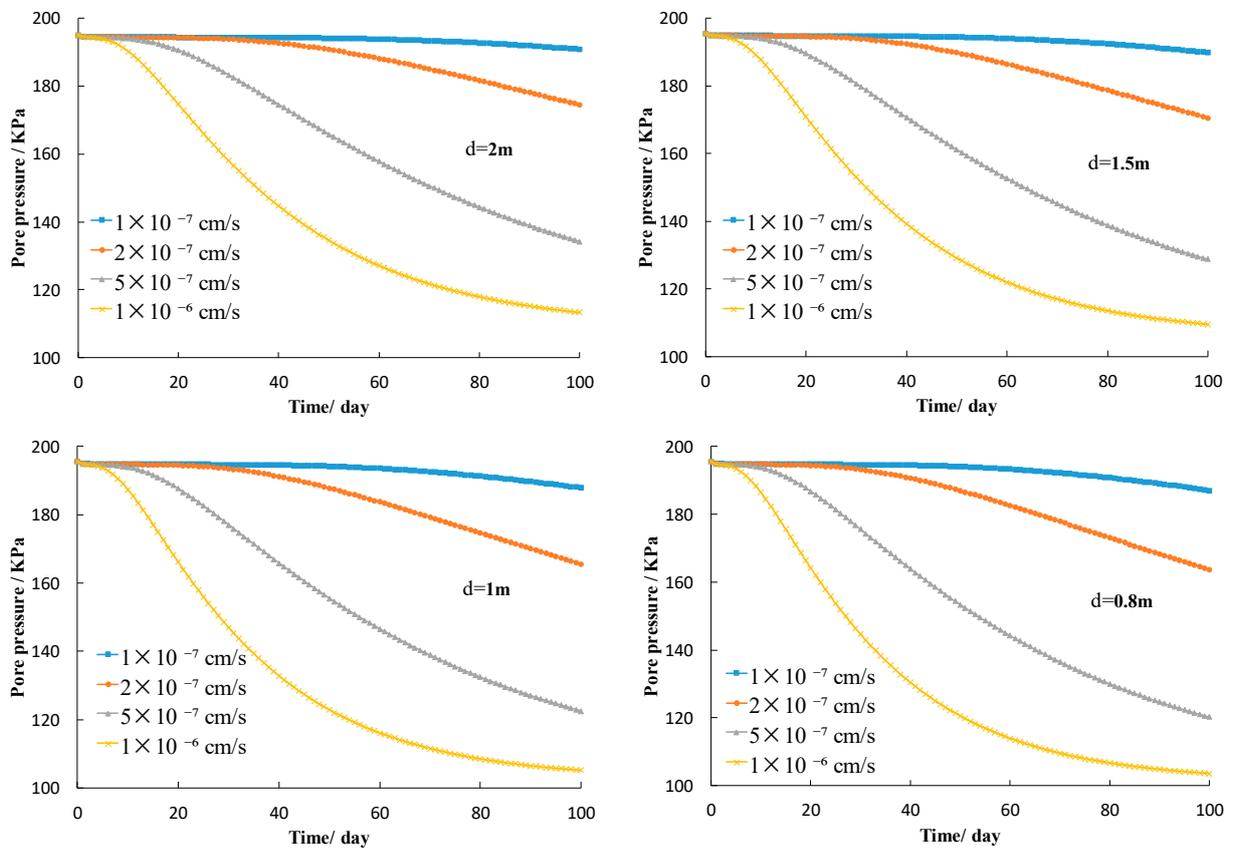
Figure 9. Pore water pressure at a depth of 20 m at the corner of the square column changes over time.
