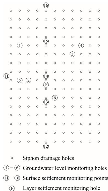
**Figure 11.** Layout of monitoring holes and points.
