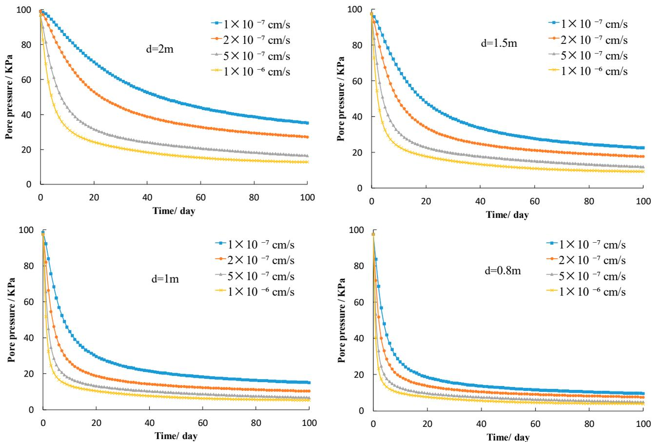
**Figure 7.** Pore water pressure at depth of 10 m at the corner of the square column changes over time.
