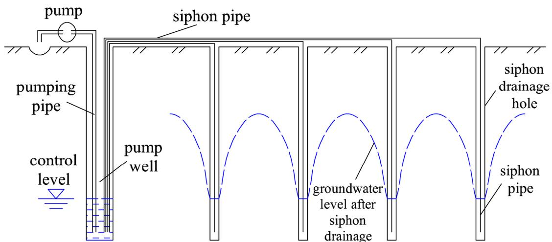
**Figure 2.** Schematic diagram of siphon drainage profile structure in soft soil.
