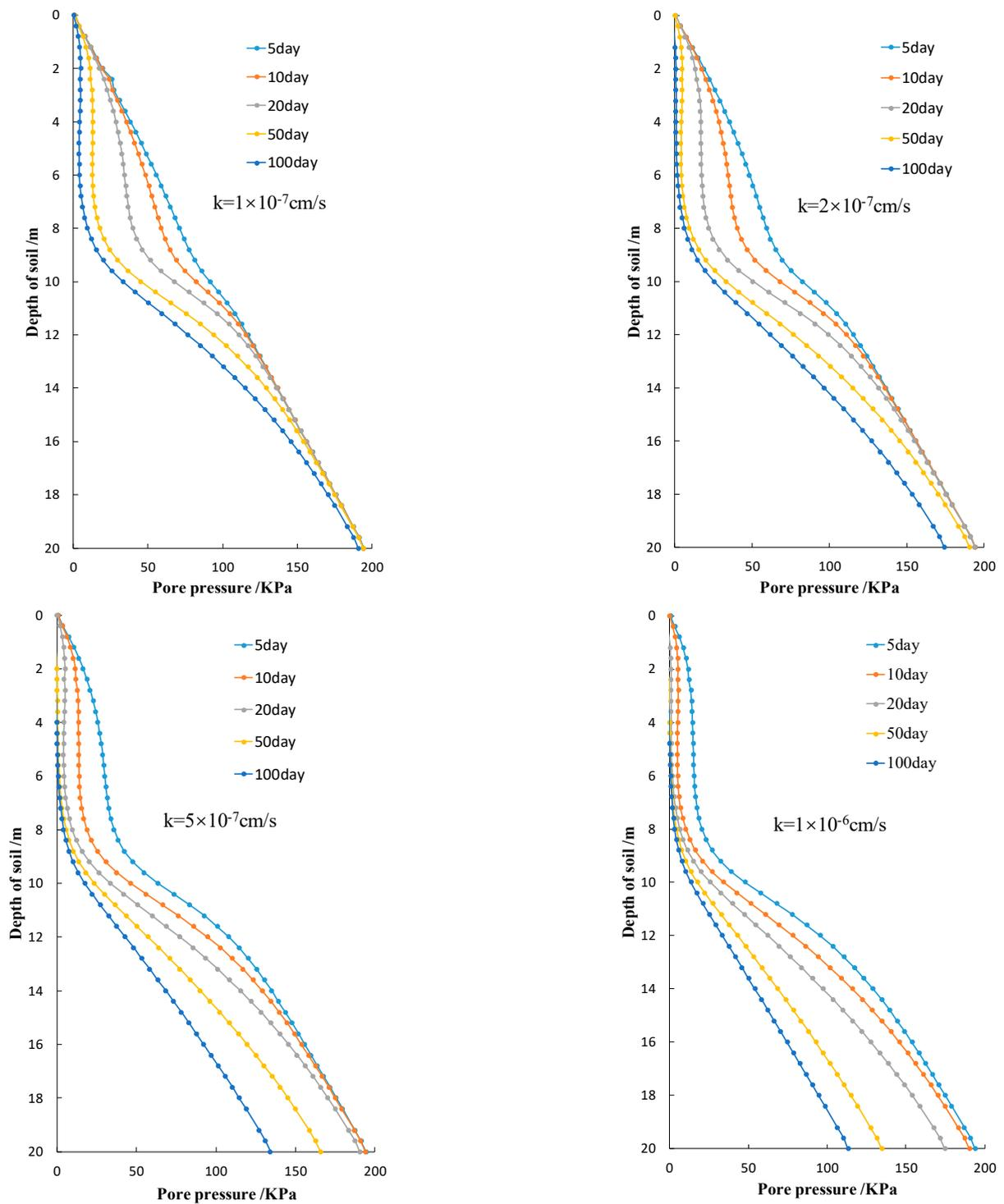
**Figure 5.** Vertical distribution of soil pore water pressure at corner of square column at siphon hole spacing  $d = 2$  m.
