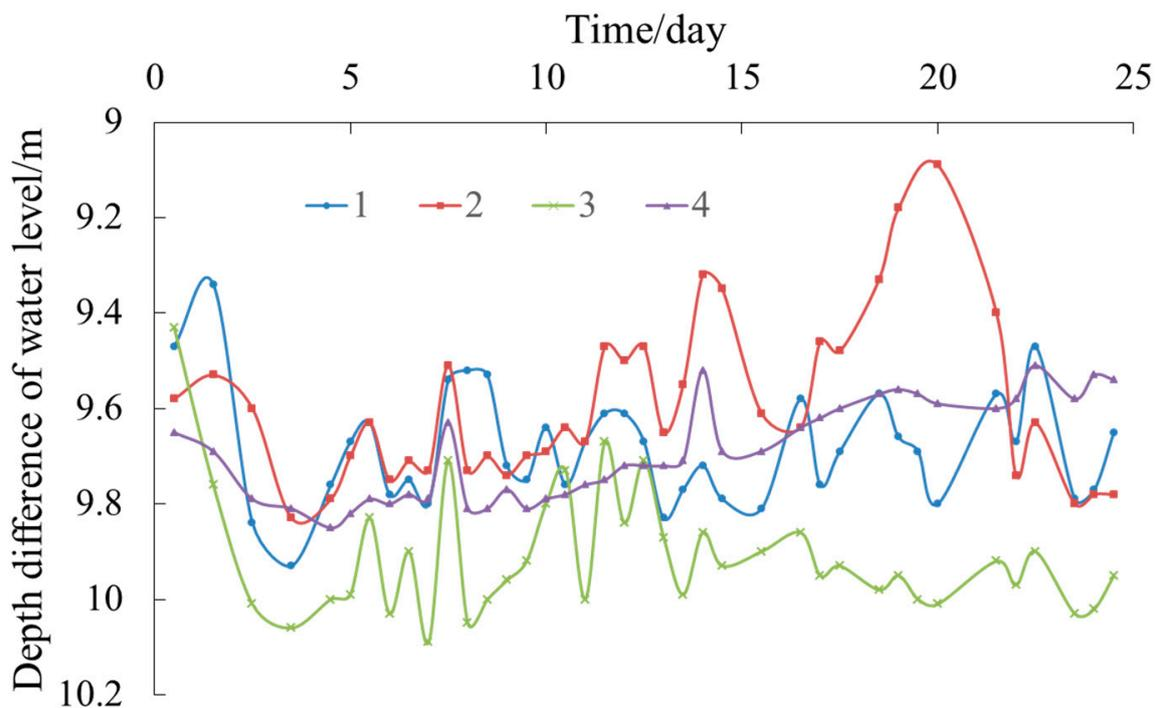
Figure 13. Depth drop of water level in siphon drainage holes.
