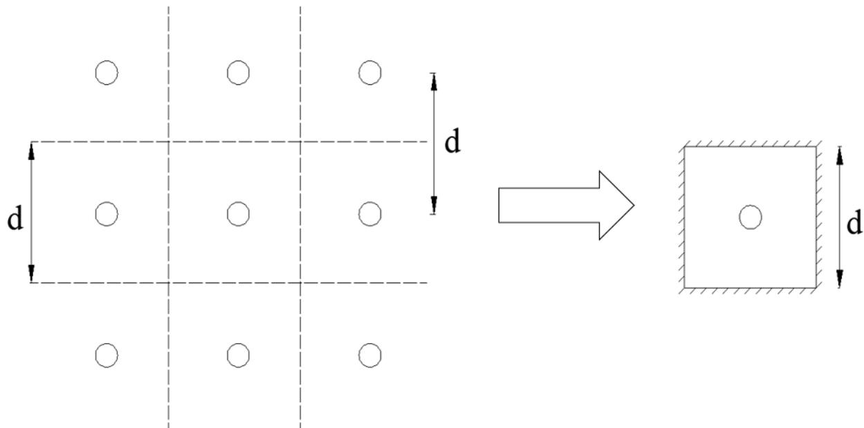
**Figure 3.** Square arrangement of siphon drainage holes.
