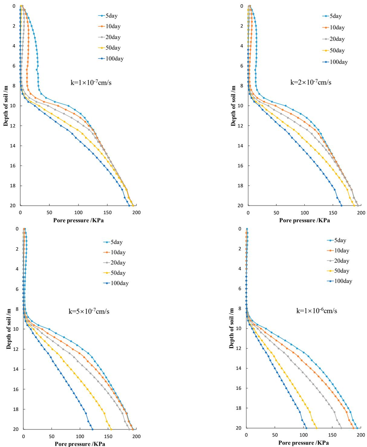
**Figure 6.** Vertical distribution of soil pore water pressure at corner of square column at siphon hole spacing  $d = 1$  m.
