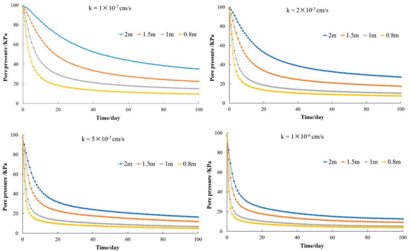
Figure 8. Pore water pressure at a depth of 10 m changes over time under different spacings.
