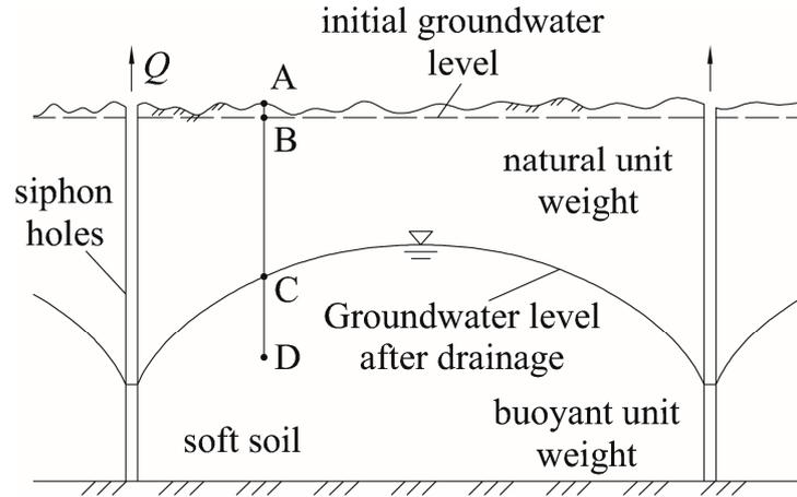
**Figure 1.** Diagram of groundwater level in soil mass before and after siphon drainage (Point A is at the surface, point B is at the initial groundwater level, point C is at the groundwater level after drainage, and point D is below the groundwater level after drainage).
