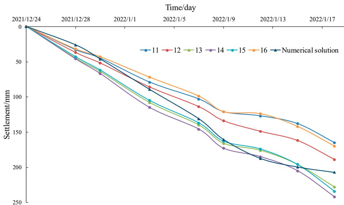
Figure 15. The surface settlement in the siphon drainage test area.
