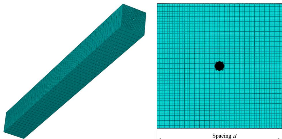
**Figure 4.** Mesh schematic of the model.
