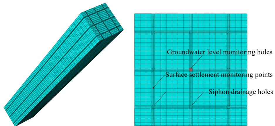
Figure 12. Mesh schematic of the numerical model.
