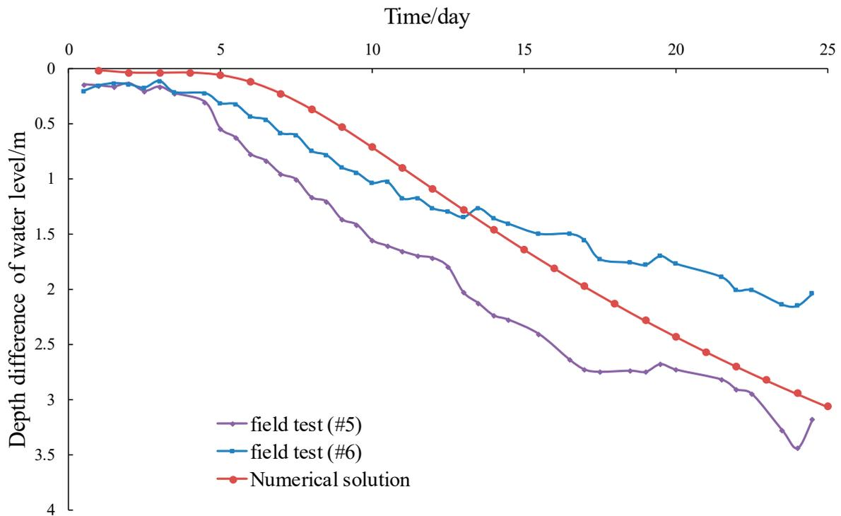
Figure 14. Water level decrease in groundwater level monitoring holes.
