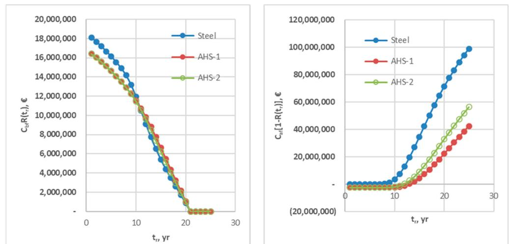
Figure 9. Cost of repair before failure (left) and after failure (right).
