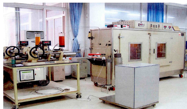
Figure 2. Core displacement system.
