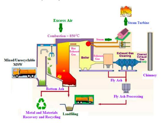
Incineration includes the following stages, as shown in Figure 2: incineration, energy recovery, and air pollution control [13].
