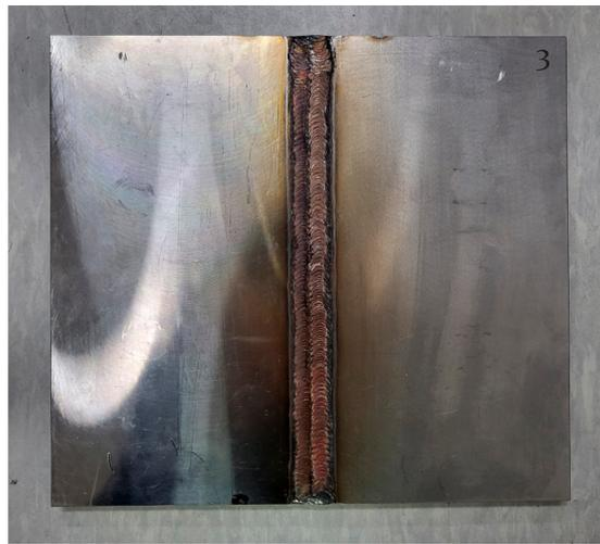
**Figure 3.** Sample of an artificial flaw specimen.
