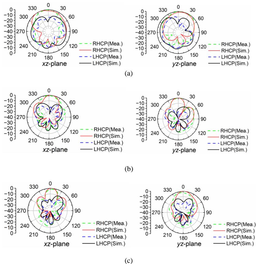
**Figure 10.** The simulated and measured radiation patterns of the proposed antenna at (a) 3.0 GHz, (b) 4.0 GHz, and (c) 5.0 GHz.
