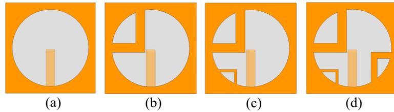
**Figure 2.** Four reference prototypes in the design process of circular slot antenna. (a) Ant.1. (b) Ant.2. (c) Ant.3. (d) Ant.4.
