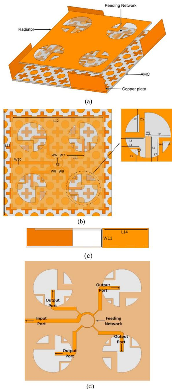
**Figure 1.** Configuration of the presented antenna. (a) 3D view. (b) Top view and detail. (c) Side view. (d) Feeding network.
