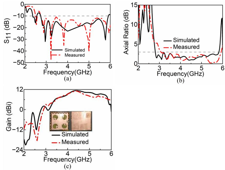
Figure 9. Simulated and measured results of (a)  $S_{11}$ . (b) AR curves. (c) Gain curves.
