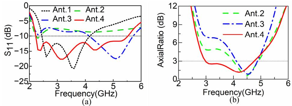
**Figure 3.**  $S_{11}$  and AR curves for different antennas. (a)  $S_{11}$ . (b) AR curves.
