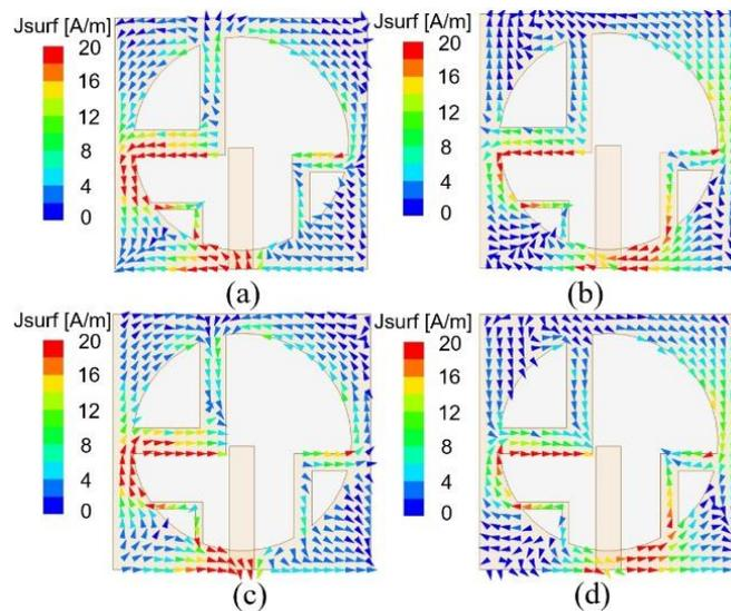
**Figure 4.** Distribution of the surface current on the antenna at 4 GHz in the phases of (a)  $0^\circ$ , (b)  $90^\circ$ , (c)  $180^\circ$  and (d)  $270^\circ$ .
