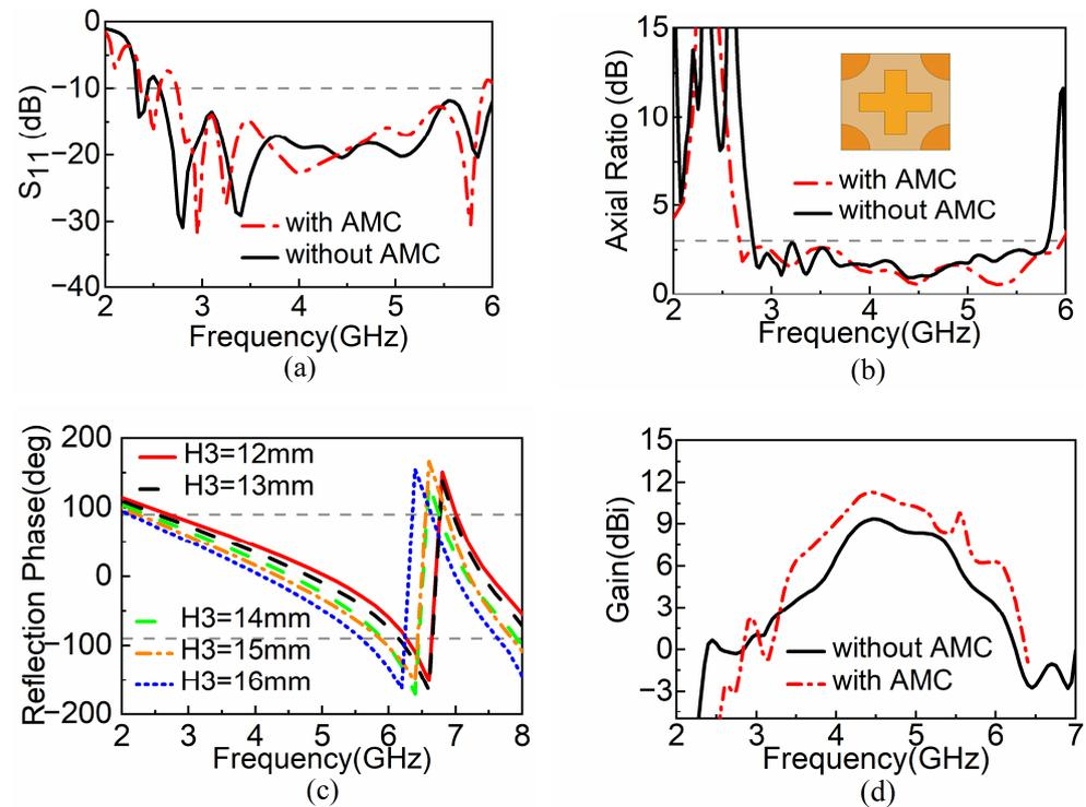
**Figure 5.** Influence of AMC structure on antenna performance and parameter scanning of air layer height. (a)  $S_{11}$ . (b) AR curves. (c) Air layer height H3. (d) Gain curves.
