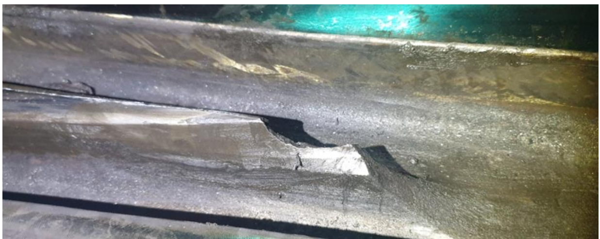
Figure 7. Partial fracture of the nose.
