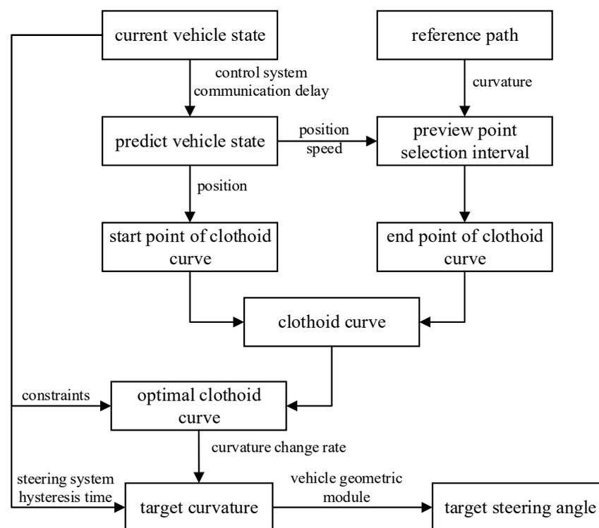
**Figure 1.** Clothoid-curve-based trajectory tracking control method.
