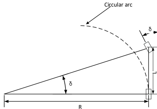
**Figure 2.** Geometric model based on Ackerman steering configuration.
