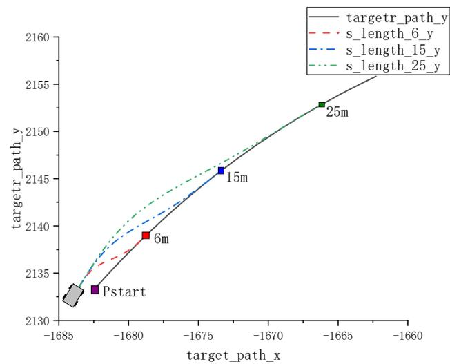
**Figure 4.** Influence of the selection of preview point on the calculation deviation of control path.
