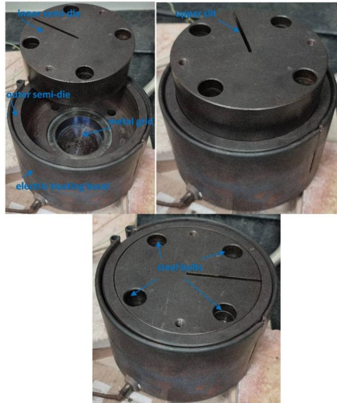
**Figure 4.** Forming die constituting two parts.
