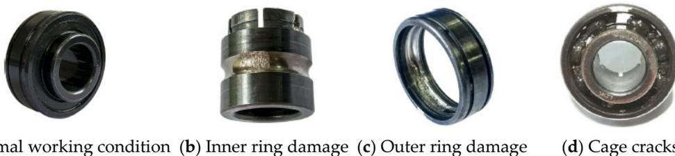
**Figure 6.** Images of typical bearing failure types.
