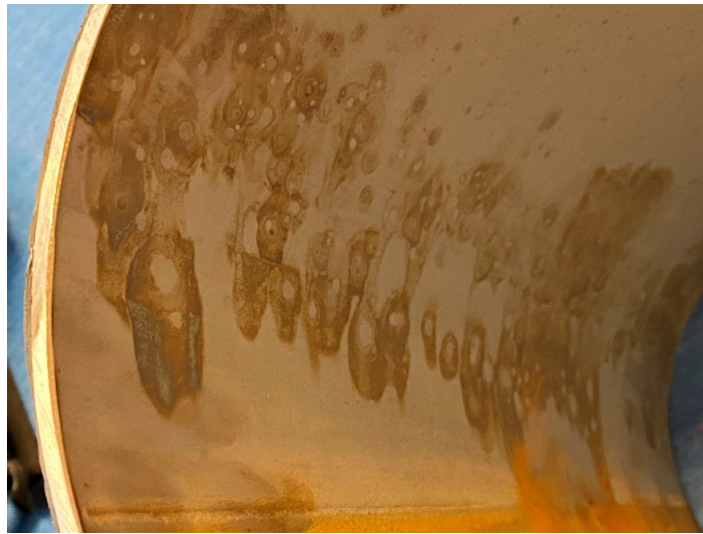
Figure 3. Multiple pitting onsets on the inside of the tube.
