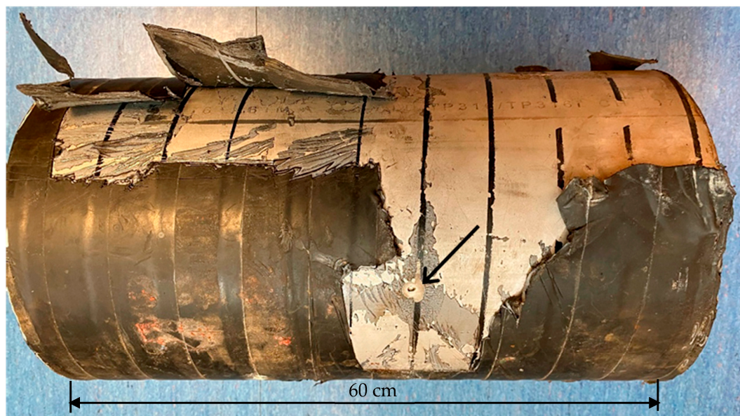
Figure 1. Sample of pipe extracted from the port piping system; a through-wall pitting can be observed in the center (black arrow).
