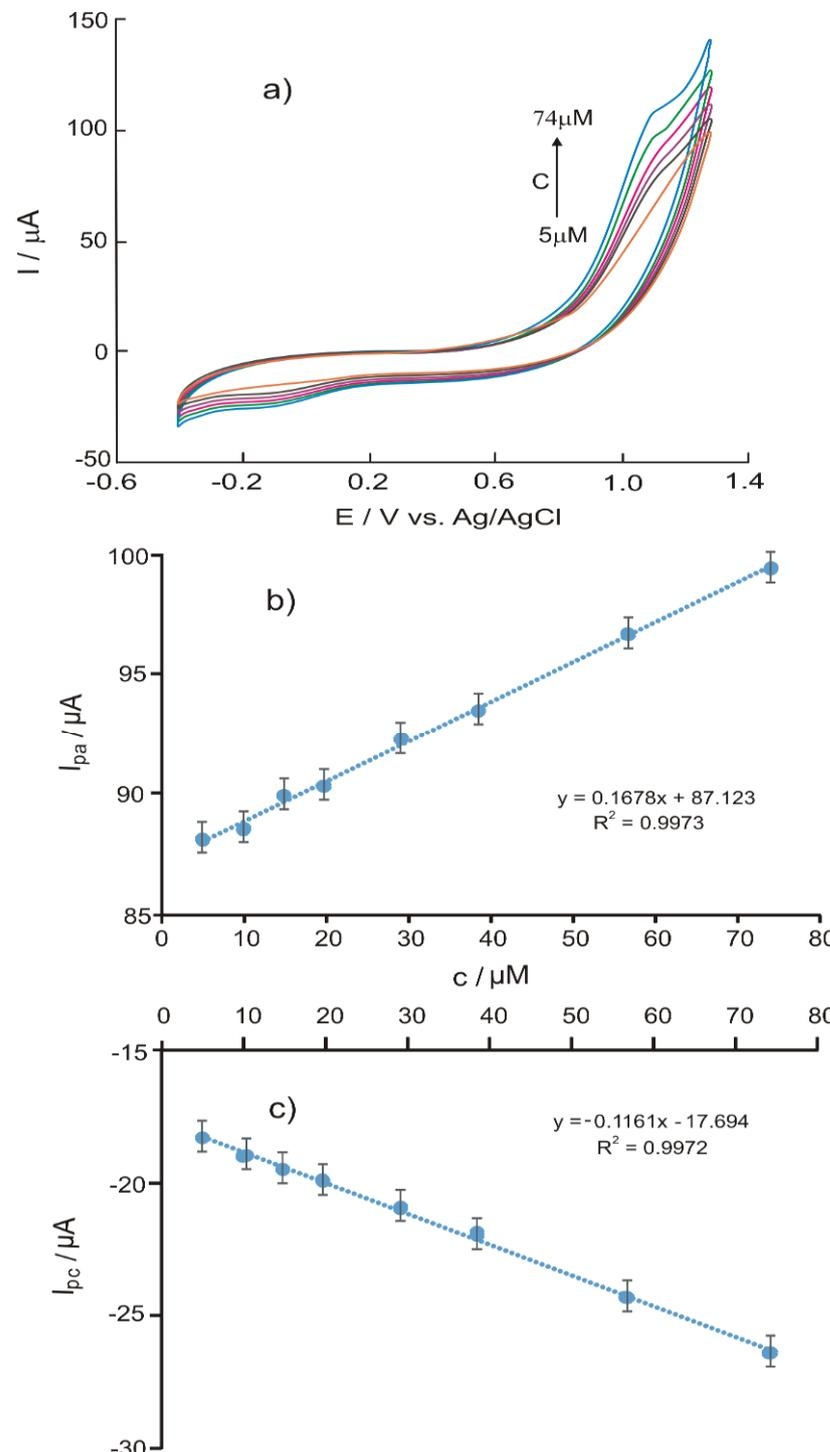
**Figure 5.** (a) Overlapping cyclic voltammograms of the SPCE/HRP biosensor, immersed in different solutions with variable concentrations of caffeic acid (electrolyte support was  $10^{-2}$  M PBS pH 7– $10^{-2}$  M hydrogen peroxide solution); (b) plot of linear calibration of the SPCE/HRP biosensor for caffeic acid based on anodic peak currents; and (c) plot of linear calibration of the SPCE/HRP biosensor for caffeic acid based on cathodic peak currents.
