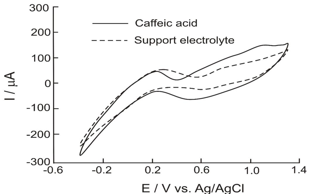
**Figure 3.** Cyclic voltammogram of SPCE/PB/HRP biosensor immersed in electrolyte support solution ( $10^{-2}$  M PBS pH 7– $10^{-2}$  M hydrogen peroxide), (dashed line); cyclic voltammogram of SPCE/PB/HRP biosensor immersed in 30  $\mu$ M caffeic acid solution in electrolyte support solution (solid line).
