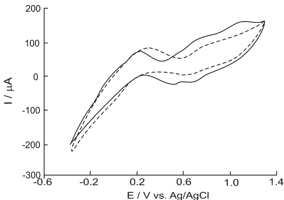
**Figure 7.** Cyclic voltammogram of SPCE/PB/HRP biosensor immersed in 20  $\mu\text{M}$  caffeic acid and 20  $\mu\text{M}$  caffeic acid solution in  $10^{-2}$  M PBS pH 7– $10^{-2}$  M hydrogen peroxide solution (solid line); cyclic voltammogram of SPCE/PB/HRP biosensor immersed in  $10^{-2}$  M PBS pH 7– $10^{-2}$  M hydrogen peroxide solution (dashed line).
