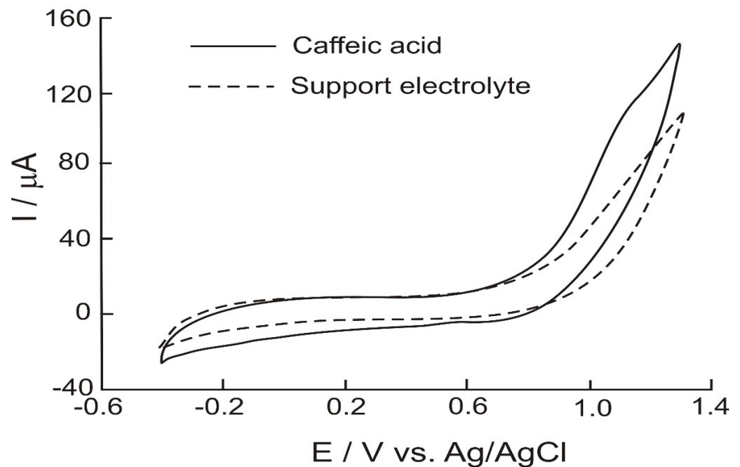
**Figure 2.** Cyclic voltammogram of SPCE/HRP biosensor immersed in electrolyte support solution ( $10^{-2}$  M PBS pH 7– $10^{-2}$  M hydrogen peroxide), (dashed line); cyclic voltammogram of SPCE/HRP biosensor immersed in 30  $\mu$ M caffeic acid solution in electrolyte support solution (solid line).
