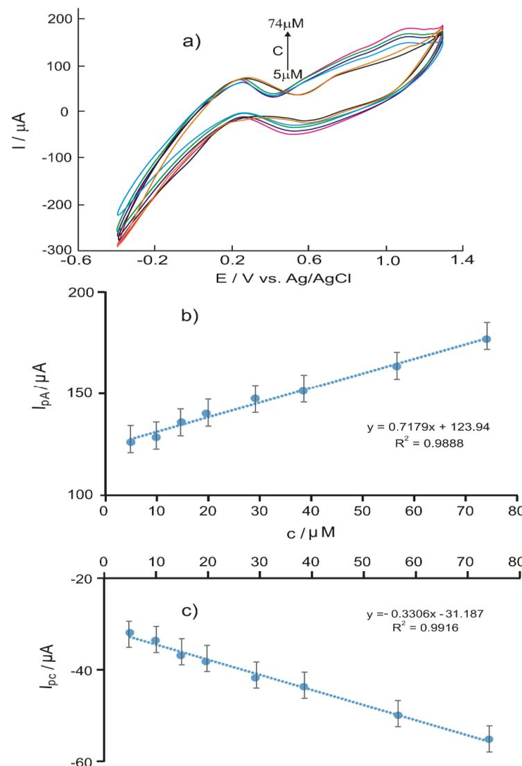
**Figure 6.** (a) Overlapping cyclic voltammograms of SPCE/PB/HRP biosensor, immersed in different solutions with variable concentrations of caffeic acid (electrolyte support was  $10^{-2}$  M PBS pH 7– $10^{-2}$  M hydrogen peroxide solution); (b) plot of linear calibration of the SPCE/PB/HRP biosensor for caffeic acid based on anodic peak currents; and (c) plot of linear calibration of the SPCE/PB/HRP biosensor for caffeic acid based on cathodic peak currents.
