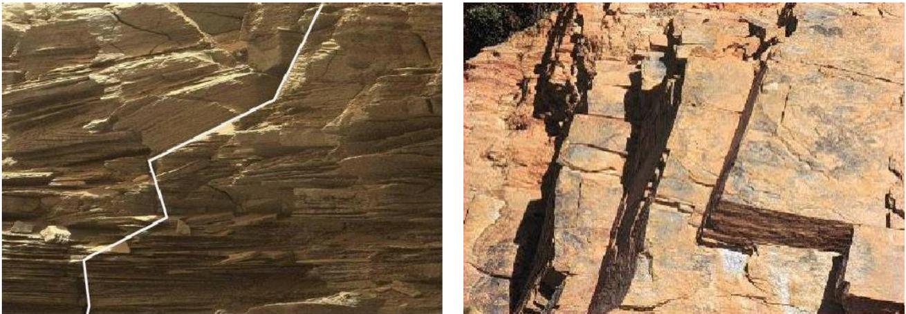
**Figure 1.** Natural irregular sawtooth rock discontinuity [7].
