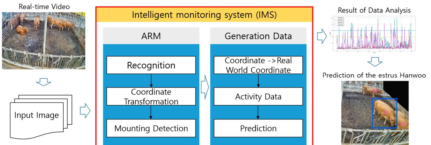
**Figure 4.** IMS structure and process with the ARM.
