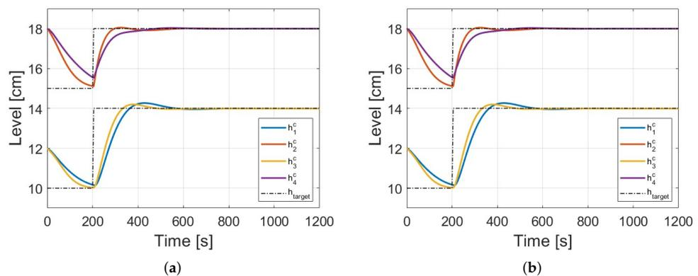
**Figure 8.** Validation Case 3: Evolution of the levels of the controlled variables involving steps: (a) Conf. 1 performance; (b) Conf. 2 performance.
