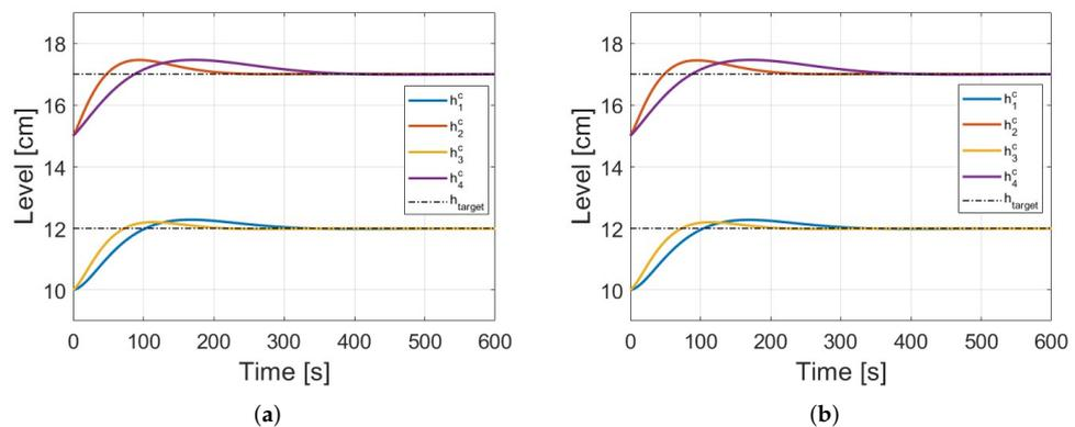
**Figure 6.** Validation Case 1: Evolution of the levels of the controlled variables: (a) Conf. 1 performance; (b) Conf. 2 performance.
