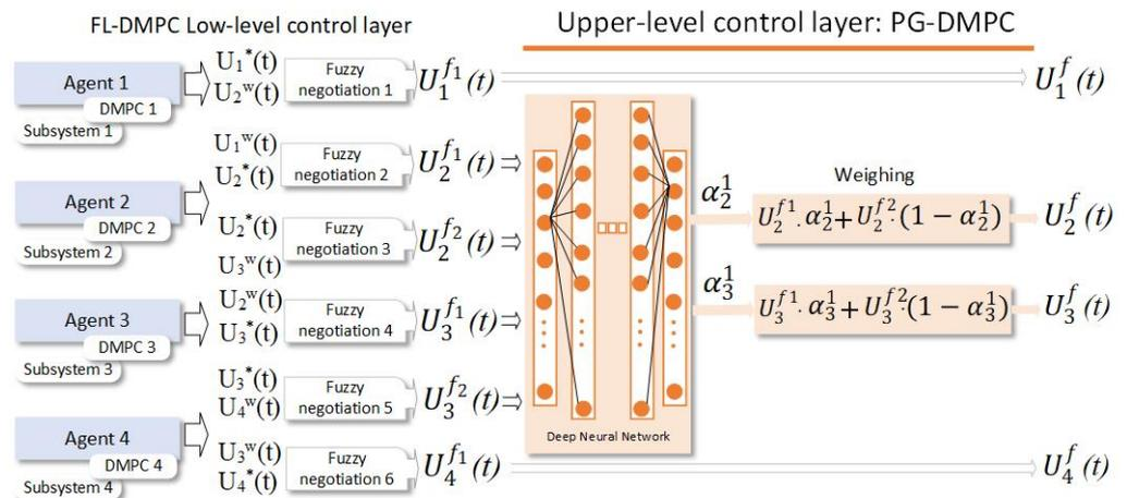
Figure 4. PG-DMPC negotiation algorithm implemented.
