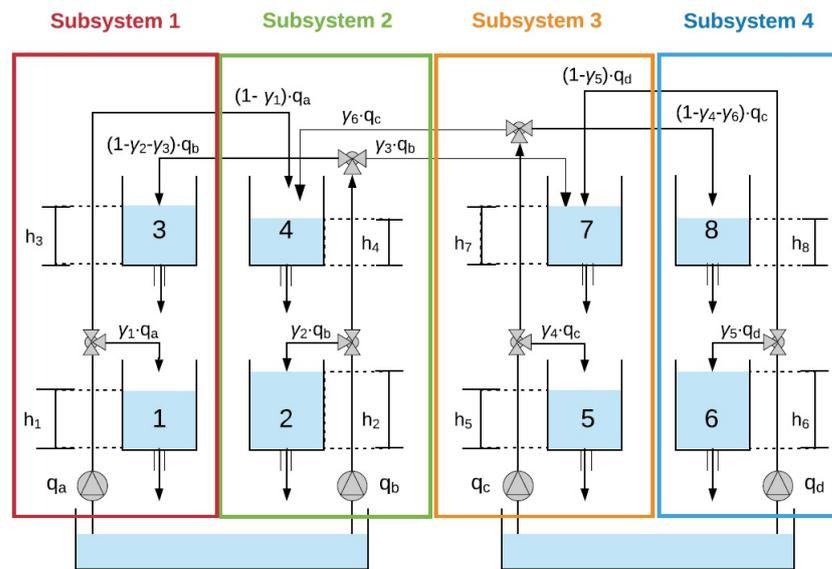
Figure 3. Schematic diagram of the eight-coupled tanks plant with the proposed subsystems.
