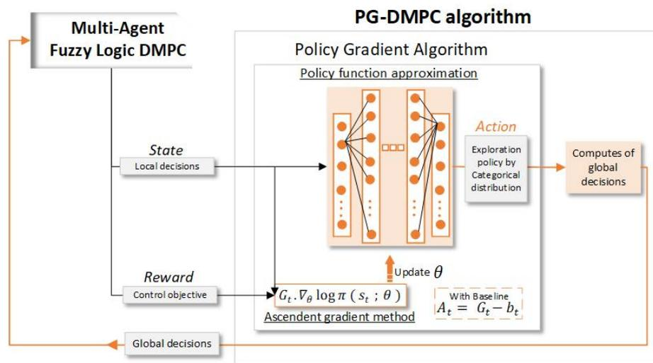
**Figure 2.** PG optimization scheme for the required negotiation agent in the upper-level control layer in the distributed MPC-based control system.
