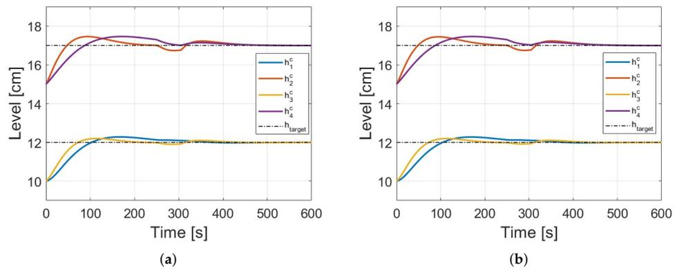
**Figure 7.** Validation Case 2: Evolution of the levels of the controlled variables involving disturbance in the state vector; (a) Conf. 1 performance; (b) Conf. 2 performance.
