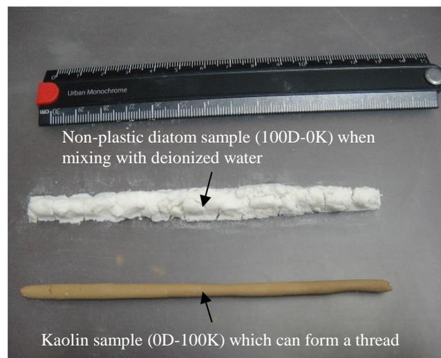
**Figure 2.** The successful case of kaolin and failed attempt of diatoms to form a thread.
