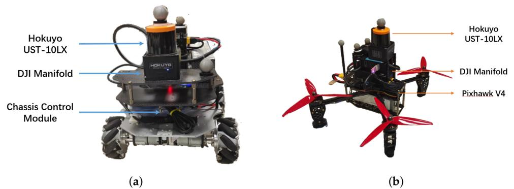
**Figure 12.** Realistic air-ground unmanned systems. (a) UGV. (b) UAV.
