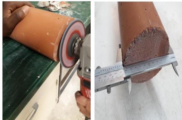
**Figure 4.** Face rectifying and measurement of cylindrical specimens.
