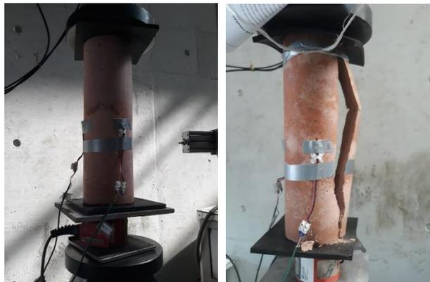
**Figure 5.** Testing and rupture of MW1 sample.
