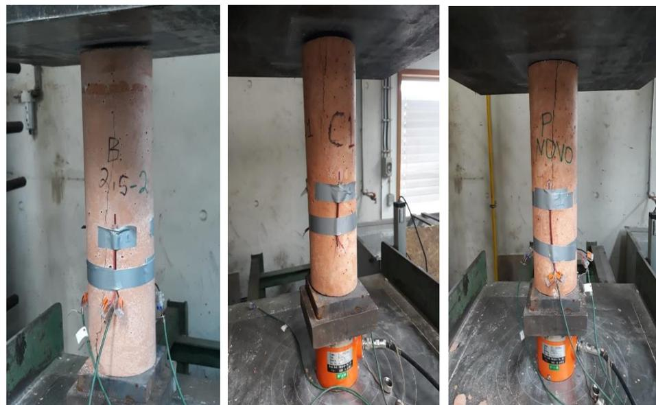
**Figure 13.** Rupture of cylinder samples in compression tests: MW2, MC, and MN.
