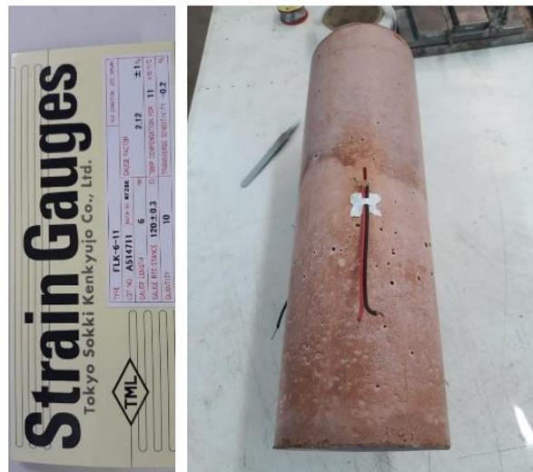
**Figure 3.** Instrumentation of cylindrical specimens.
