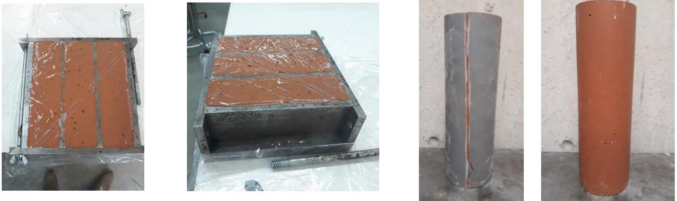
**Figure 2.** Demolding of parallelepiped and cylindrical specimens.
