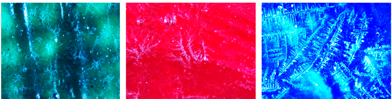
Figure 5. The optical microscopy of the metallic soap generated by the pigments.
