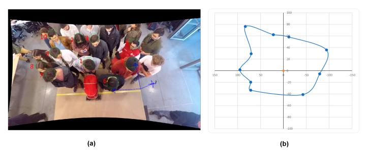
**Figure 3.** Example of the method used to identify a passenger with reduced mobility (passenger  $N^{\circ}1$ ) and those passengers around him/her (passengers  $N^{\circ}2$  to  $N^{\circ}10$ ): (a) passenger  $N^{\circ}1$  (pushing a pram) surrounded by 9 passengers (passengers  $N^{\circ}2$  to  $N^{\circ}10$ ); (b) dimensions in cm of the area used by the passenger  $N^{\circ}1$ , who is located at (0,0).
