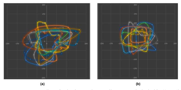
**Figure 4.** Bound graph represent the space used by a passenger with reduced mobility: (a) user with a pram; (b) wheelchair user. Coordinates are in cm.
