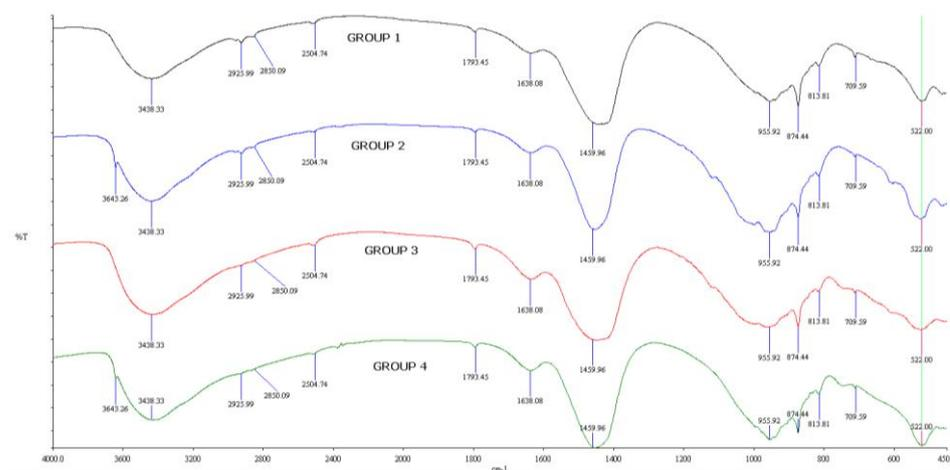
**Figure 1.** FTIR spectra of different types of cured Biodentin showing the absorbance peaks of the precipitates of each modified biodentin. Absorbance peaks ranging from 474.63  $\text{cm}^{-1}$  to 3643.26  $\text{cm}^{-1}$  are seen.
