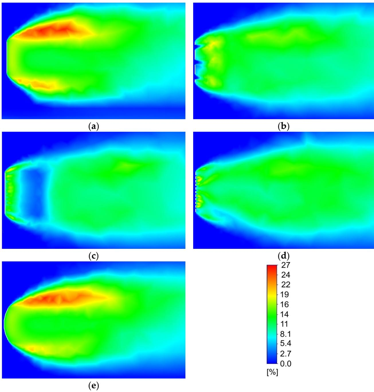
**Figure 8.** Contours of turbulence intensity around: (a) standard panel, (b) 28 staggered holes, (c) 200 uniform square holes, (d) 10 rectangular slots, and (e) curved.
