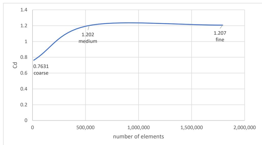
**Figure 4.** Drag coefficient ( $C_d$ ) plot for coarse, medium, and fine meshes (three meshes).
