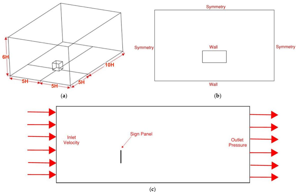
**Figure 1.** Computational domain: (a) domain dimensions for an object with height  $H$ , (b) wall and symmetric boundary conditions, and (c) inlet and outlet boundary conditions.
