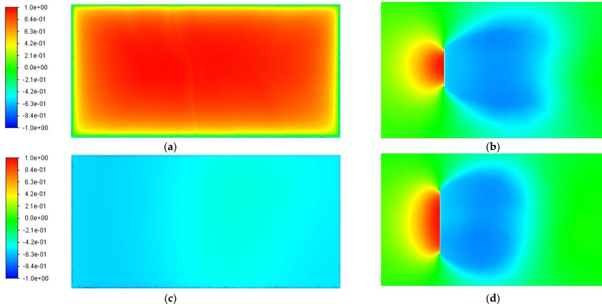
**Figure 5.** Pressure coefficients contour on the standard panel: (a) windward face, (b) side view, (c) leeward face, and (d) top view.
