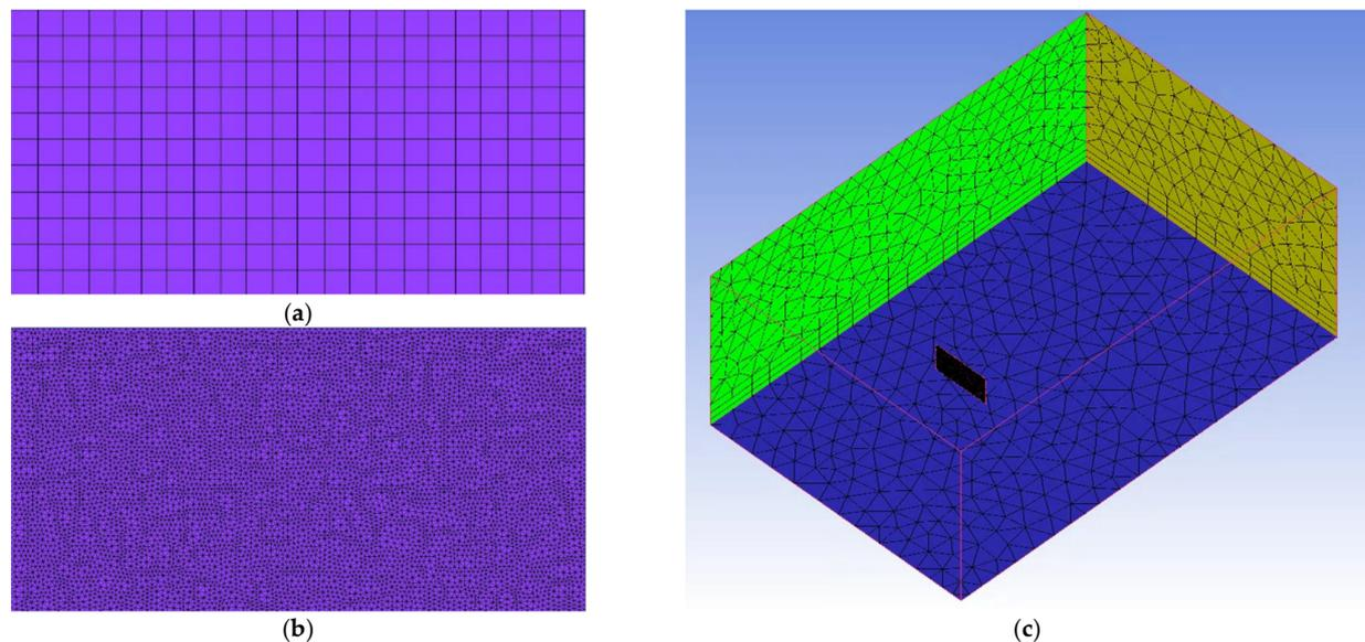
**Figure 3.** Different mesh types are employed: (a) hexahedral surface meshing of the standard sign panel, (b) tetrahedral meshing of the standard sign panel, and (c) tetrahedral surface meshing of the whole domain (coarse).
