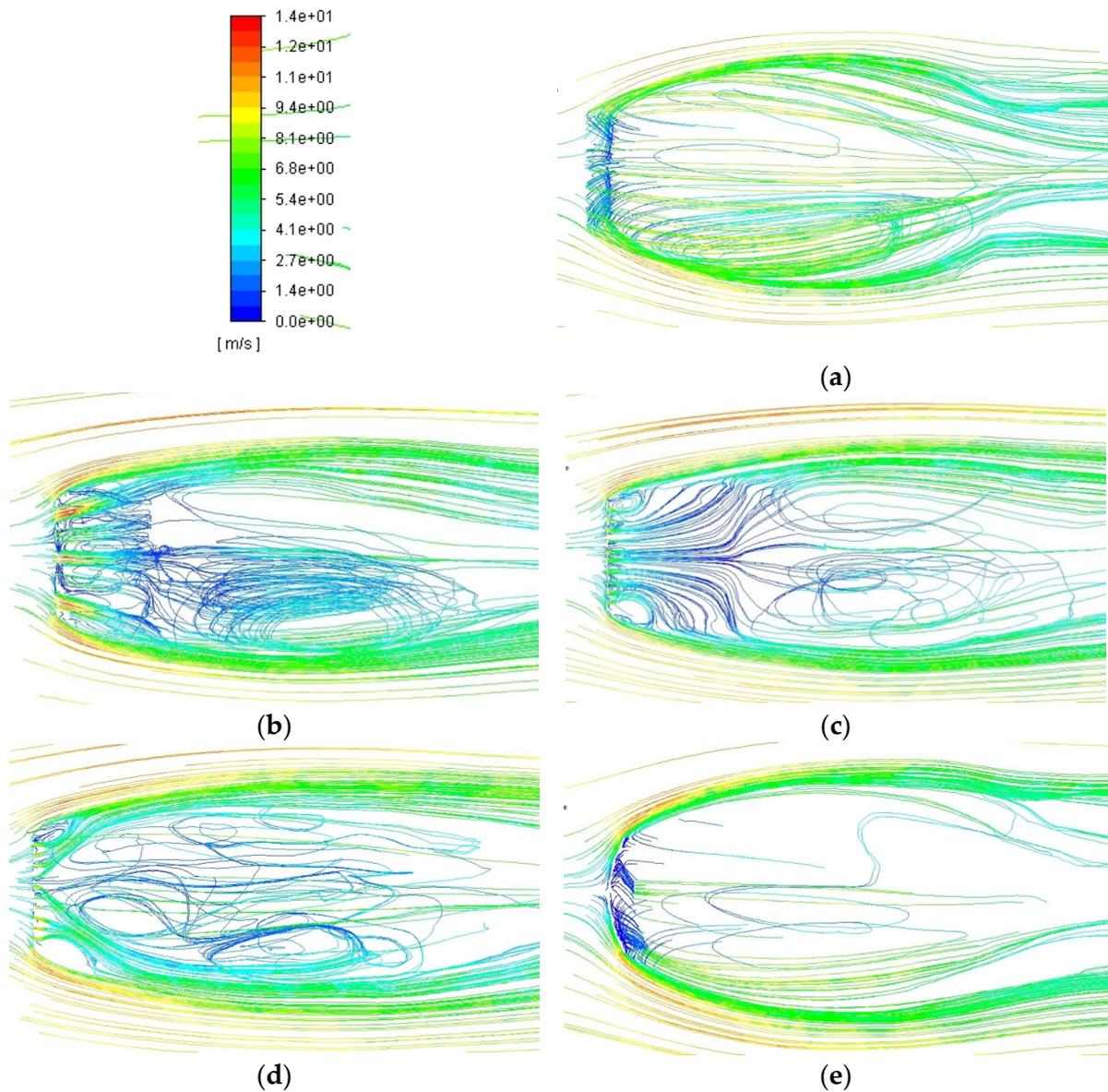
**Figure 9.** Path lines of airflow around: (a) standard panel, (b) 28 staggered holes, (c) 200 uniform square holes, (d) 10 rectangular slots, and (e) curved.
