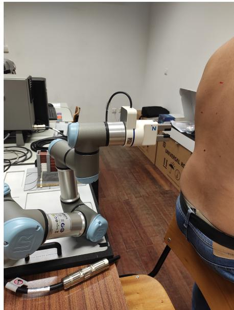
**Figure 21.** Collision of the robotic arm elbow joint with the bench where it is installed, when trying to reach the point  $L4$  of patients 2 and 4.
