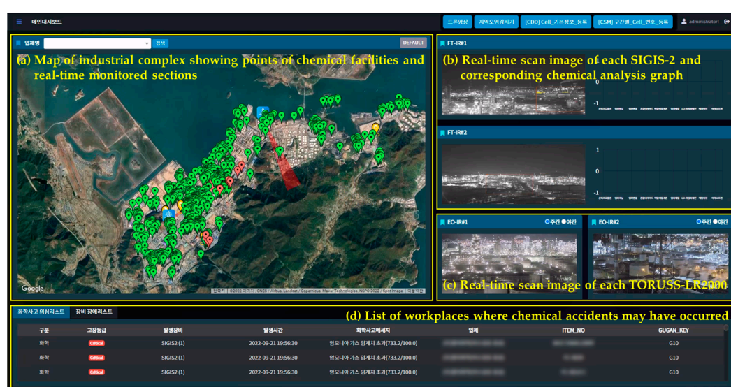
Figure 8. Main screen of the monitoring software. (a) Map of industrial complex showing points of chemical facilities and real-time monitored sections. (b) Real-time scan image of each SIGIS-2 and corresponding chemical analysis graph. (c) Real-time scan image of each TORUSS-LR2000. (d) List of workplaces where chemical accidents may have occurred.
