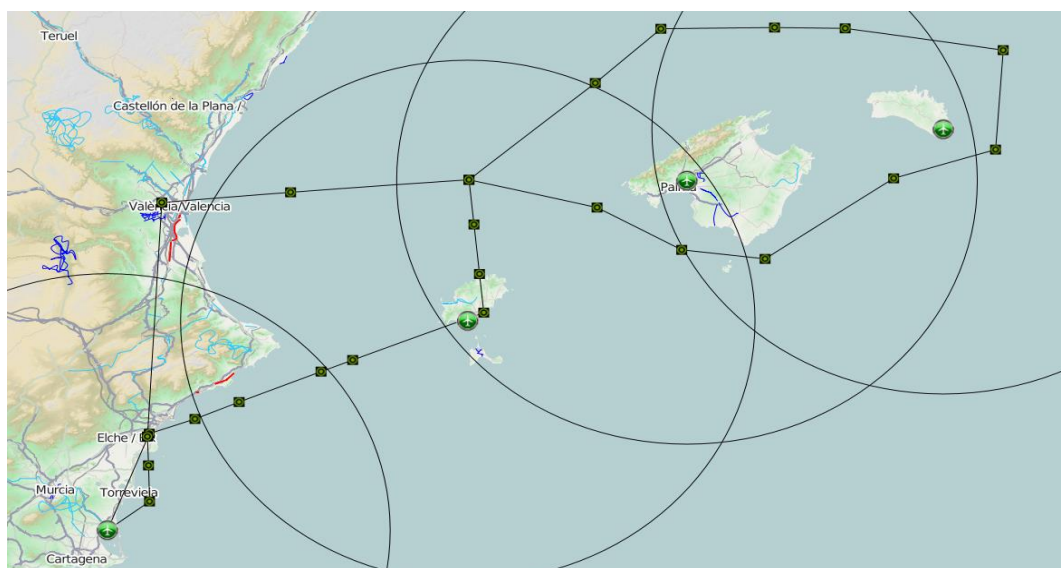
Figure 2. Emergency airfield selected for an MQ-9 RPAS engine failure contingency. Circles indicate maximum MQ-9 gliding distance (estimated around 90 NM) from mission cruise altitude.
