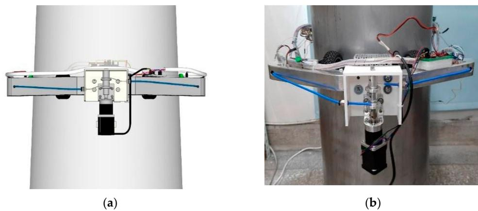
Figure 15. Body Frame 1: (a) CAD design and (b) actual physical view.
