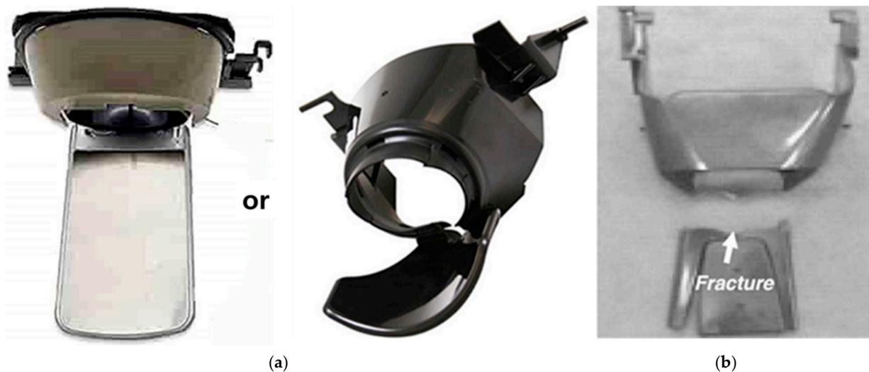
**Figure 8.** Damaged dispenser lever after usage. (a) Water dispenser and (b) failed dispenser lever in the field.
