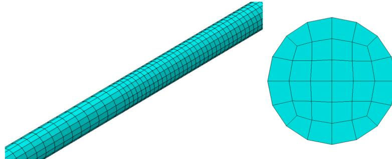
**Figure 5.** Overall mesh of the bolt (left); cross-section of the bolt (right).
