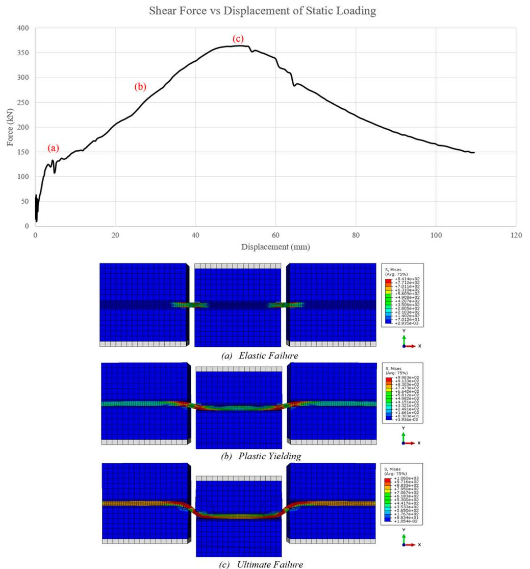
Figure 13. Three stages of bolt failure under static loading conditions.
