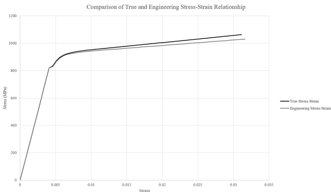
**Figure 3.** Engineering vs. true stress–strain curve.
