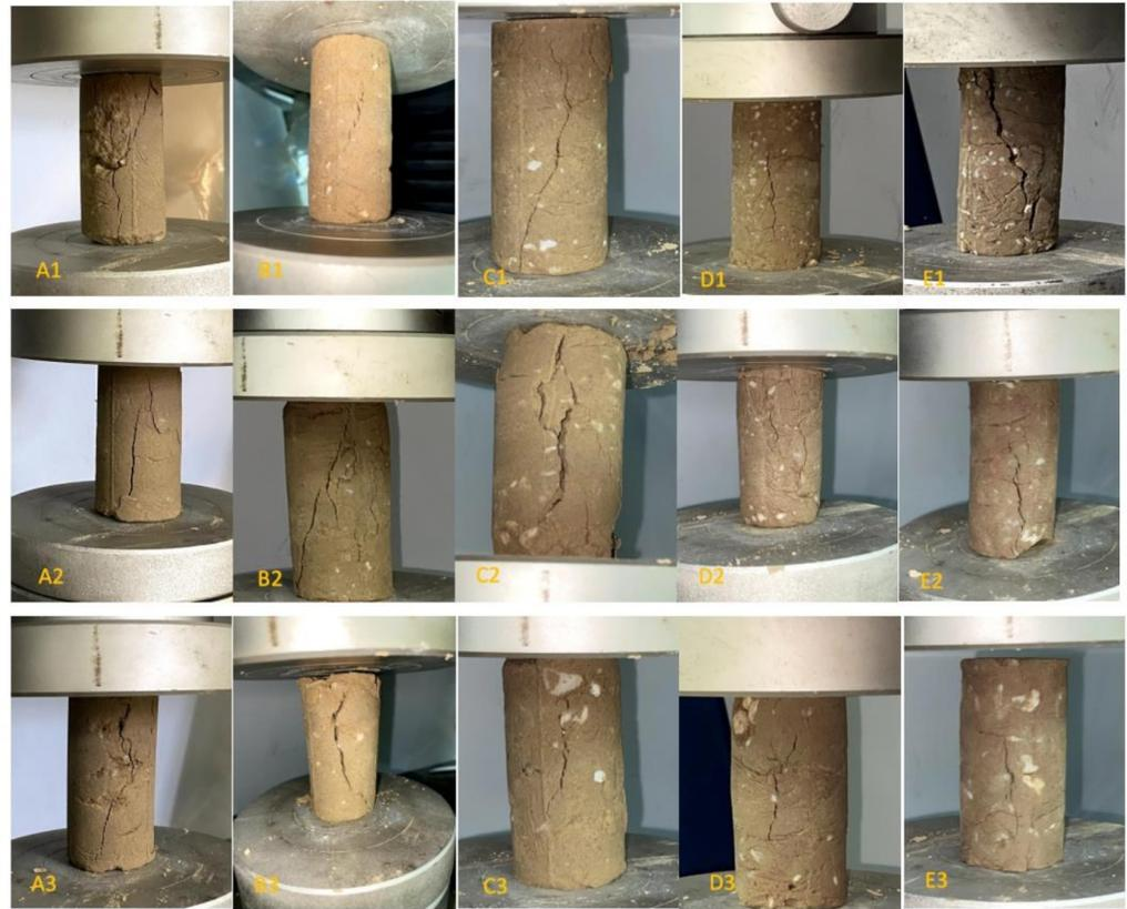
**Figure 2.** Results of unconfined compression test of soil–rock mixture (See Table 2 for the sample corresponding to each letter).
