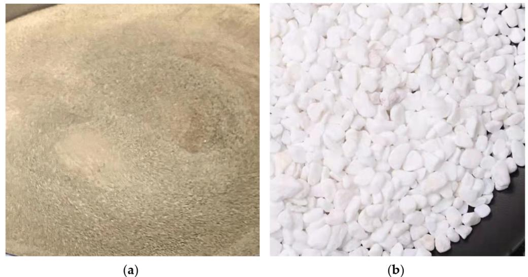
**Figure 1.** Raw material of soil–rock mixture: (a) silt, (b) rock.
