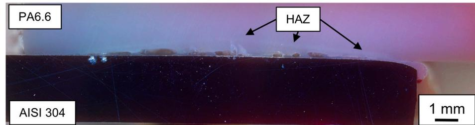
**Figure 9.** Cross-section of a cold-rolled AISI 304–Polyamide 6.6 (PA6.6) hybrid joined with  $158 \text{ J mm}^{-1}$  with visible pores and the heat affected zone (HAZ).
