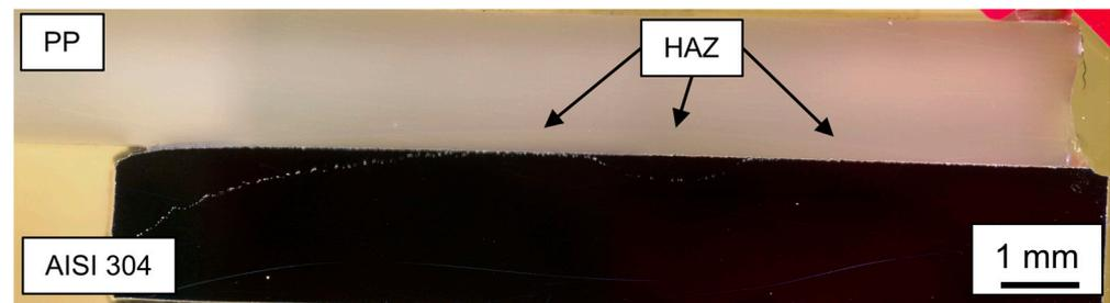
**Figure 13.** Cross-section of a sandblasted AISI 304–polypropylene hybrid joined with  $81 \text{ J mm}^{-1}$ .
