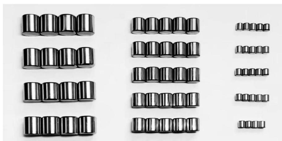
**Figure 9.** Cylindrical roller specimens.
