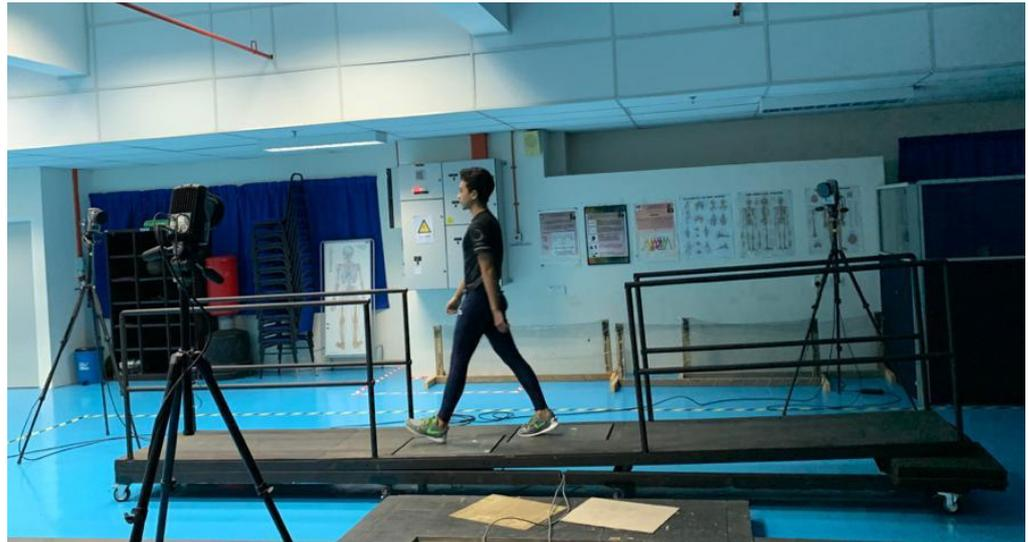
**Figure 3.** Illustration of subject walking downward on the customized slope platform.
