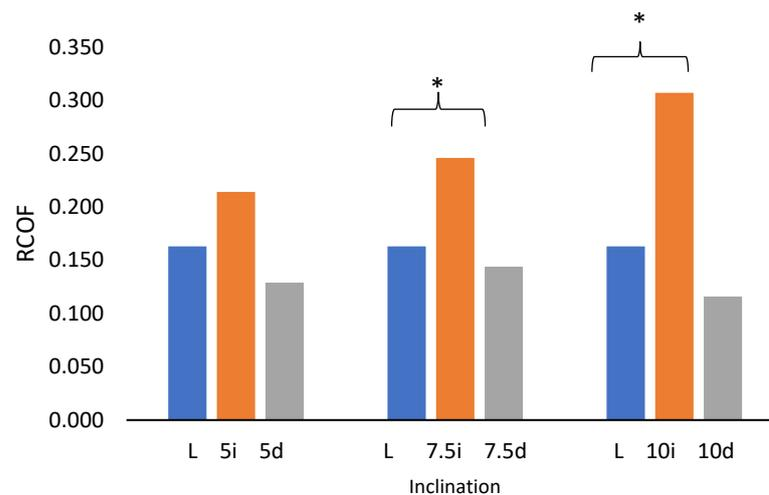
**Figure 7.** Comparison of the RCOF between level and slope walking during peak GRF. Note: L = level walking; 5i, 7.5i, 10i = inclined walking of 5°, 7.5°, 10°; 5d, 7.5d, 10d = decline walking of 5°, 7.5°, 10°; \* = significant difference compared between level and inclined walking.
