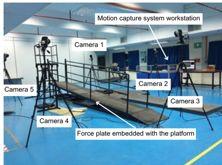
Figure 1. Equipment set-up.
