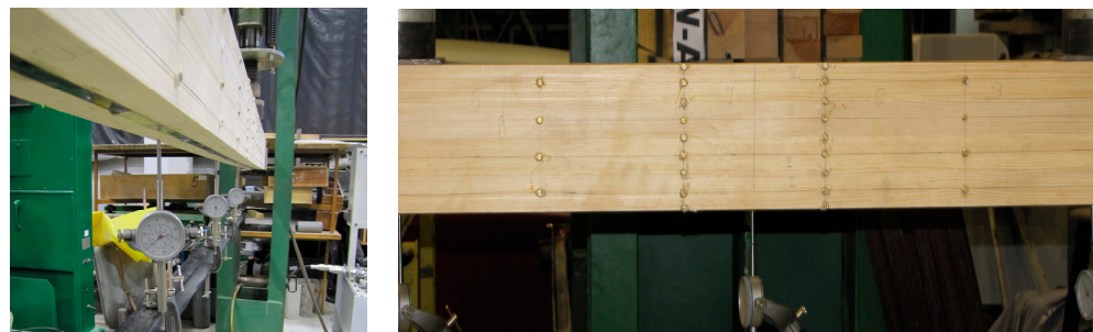
Figure 3. The distribution of the placement of the inductive sensors along the 5h and the bases for the strain measurements along the length of the beams.
