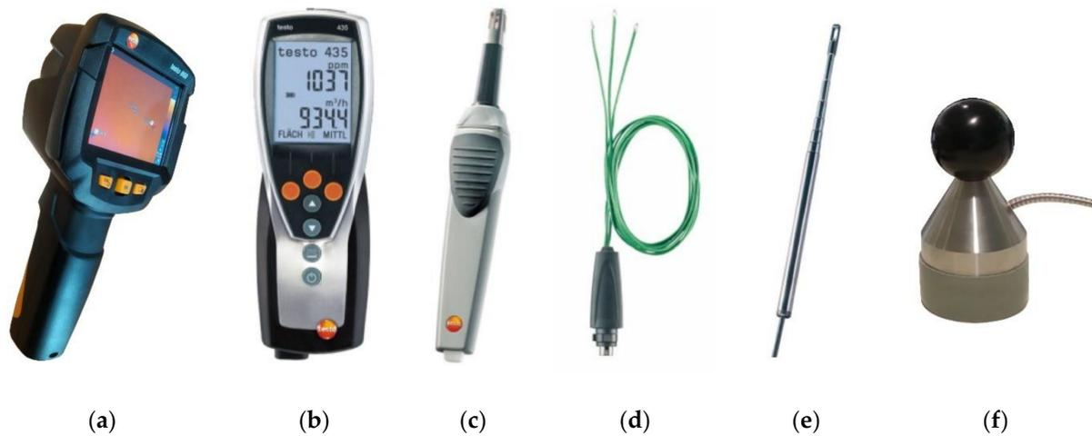
**Figure 5.** Measuring devices: (a) thermographic camera; (b) thermal transmittance flowmeter; (c) humidity/temperature probe; (d) surface probe; (e) hot wire probe; and (f) black balloon probe.
