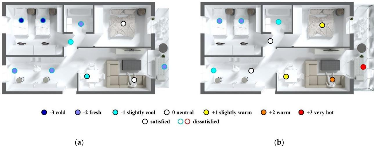
**Figure 9.** Comfort survey results in the coldest week of the year (3–7 January): (a) without a “glass curtain” system and (b) with a “glass curtain” system closed.
