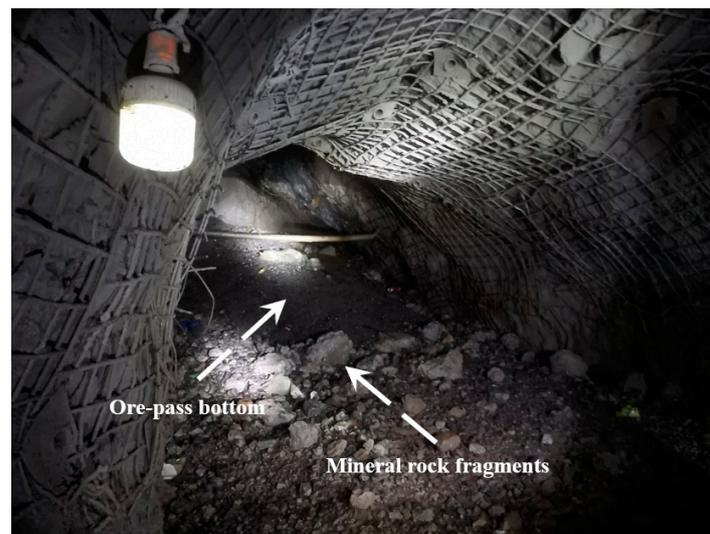
Figure 7. Bottom of No. 2 ore pass of the deep mine.
