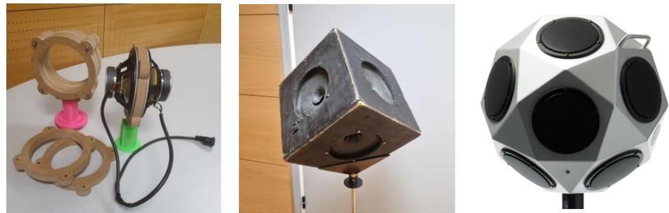
**Figure 1.** Omnidirectional sound sources used in the research—the coupled speakers (**left**), cubic omnidirectional sound source (**middle**), and dodecahedral omnidirectional sound source (**right**) [32].
