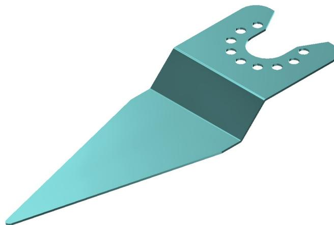
**Figure 4.** The designed shape of the tapered cutting blade consisting of one piece.
