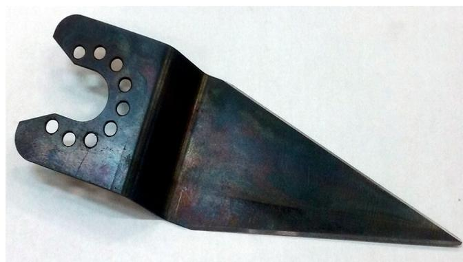
**Figure 13.** The cutting blade of the oscillating cutter made by the designed bending tool.
