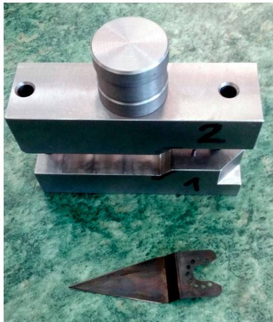
**Figure 12.** Bending tool for the production of the cutting blades of the oscillating cutter (**top**) and a part made by it (**bottom**).
