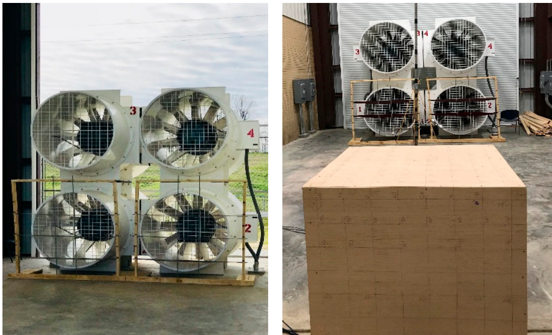
Figure 4. LSU WISE large-scale testing facility, featuring a test section measuring 4 m by 4 m.
