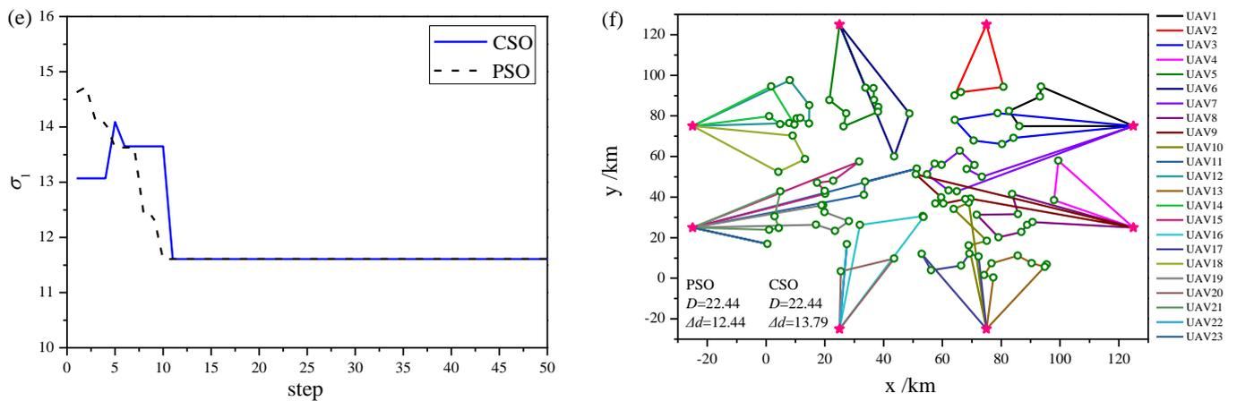
**Figure 5.** Optimization process. (a) Fitness. (b) Number of UAVs. (c) Mean length. (d) Max length. (e) Standard deviation. (f) Result. The green circle represents the target, and the pink star represents the start point.
