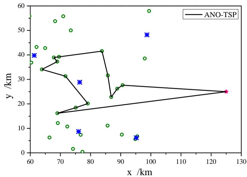
**Figure 3.** ANO–TSP path plan in cluster. The green circle represents the target, the blue symbol represents the center of clustering, and the pink star represents the start point.
