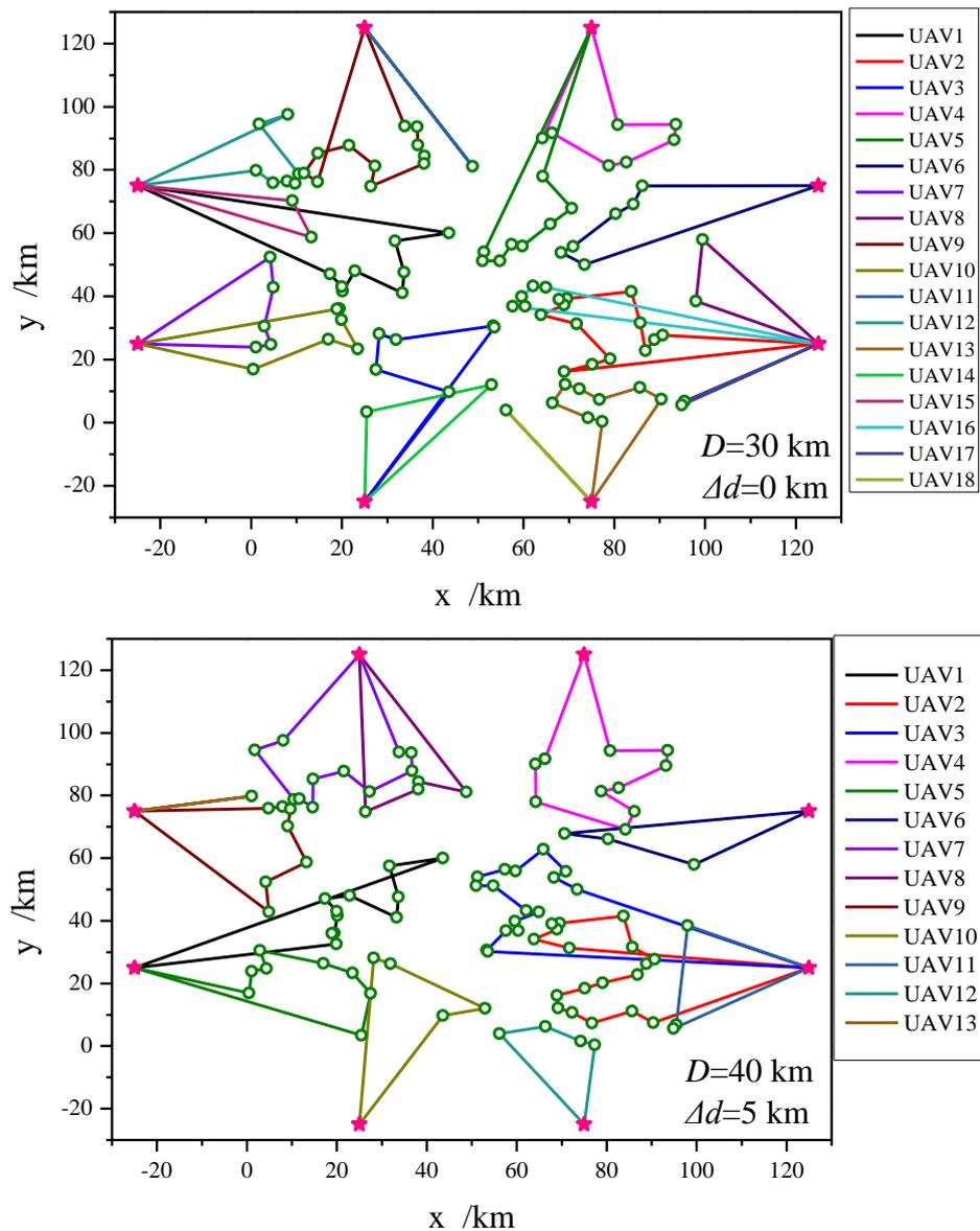
**Figure 4.** UAVs' path plan before optimization. The green circle represents the target, and the pink star represents the start point.
